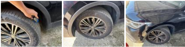
Tyre FR, Out of tolerance, Replace
