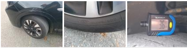
Tyre RL, Out of tolerance, Replace
