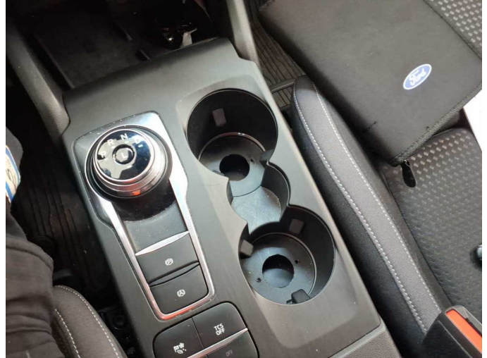
Damage 6: Instrument panel: Centre console - front ((Fehlbohrung)) - Differs from the original configuration - Replace
