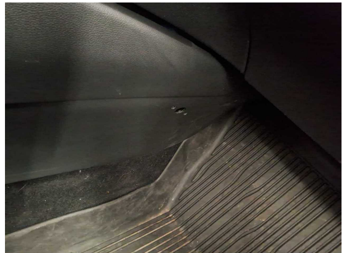
Damage 3: Instrument panel: Centre console - front (Blende vorne rechts) - Differs from the original configuration - Replace
