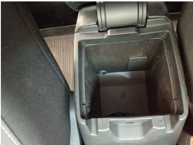
Damage 2: Interior: Arm rest, front (Deckel Hinten) - Differs from the original configuration - Replace
