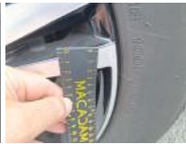
Tyre FL, Worn, Check
