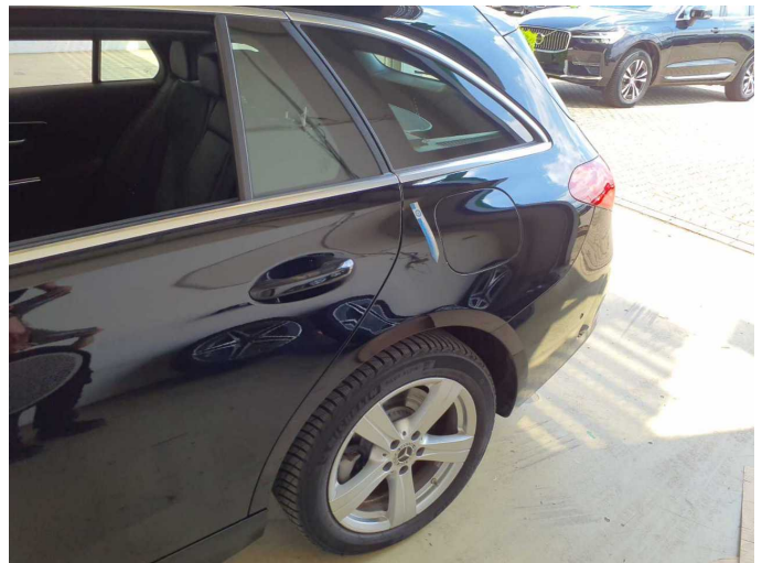
Damage 1: Side panel - rear left side: Side panel - dent(s) - Smart repair
