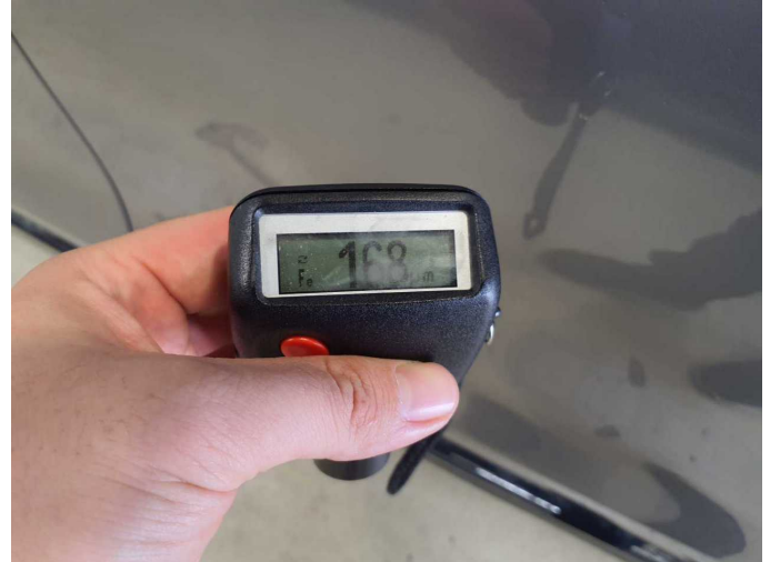
Repainting 2: Door - rear left side
