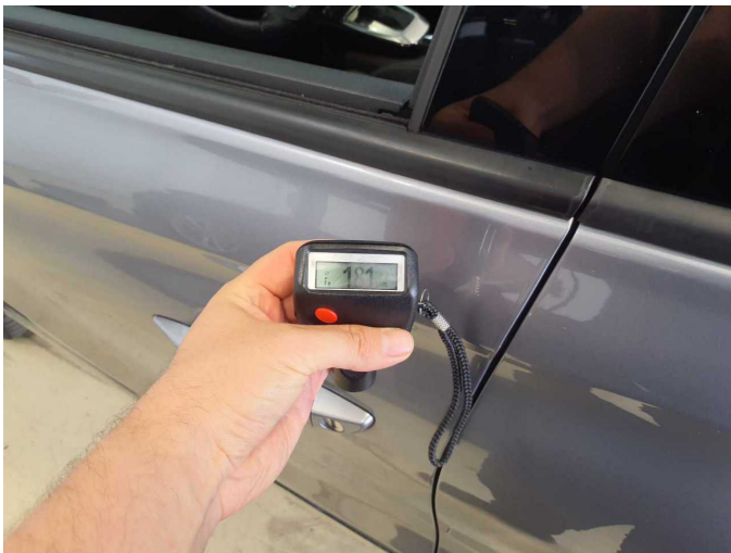
Repainting 3: Door - front left side
