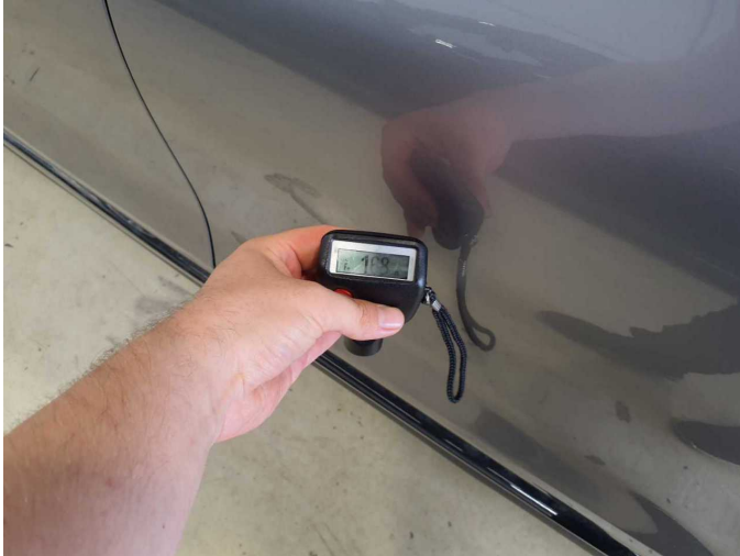
Repainting 2: Door - rear left side
