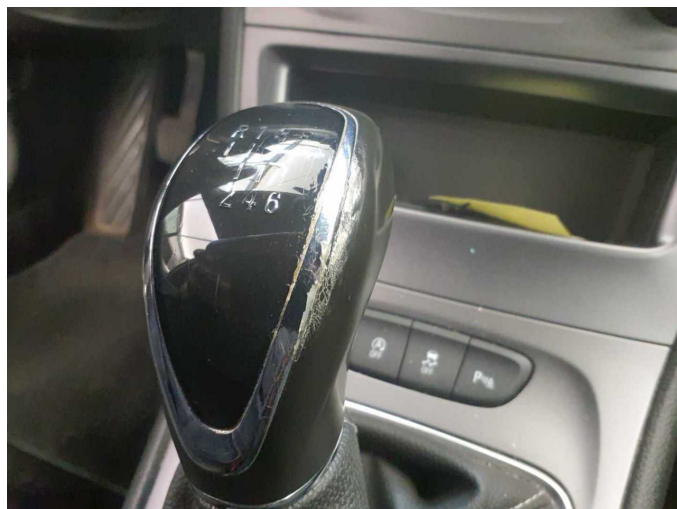
Damage 6: Gearbox: Gear knob - Abrasion - Loss in value
