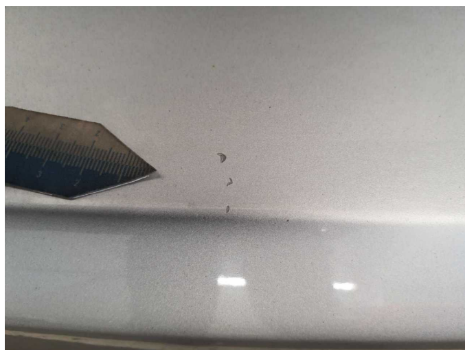
Damage 9: Rear bumper: Rear bumper - Scratch(es) - Smart repair
