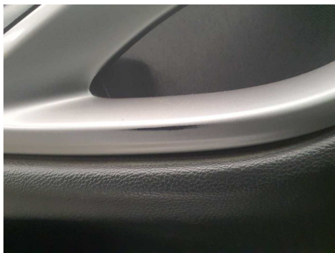
Damage 5: Door - front left side: Door handle - inside - Paint defect - Loss in value
