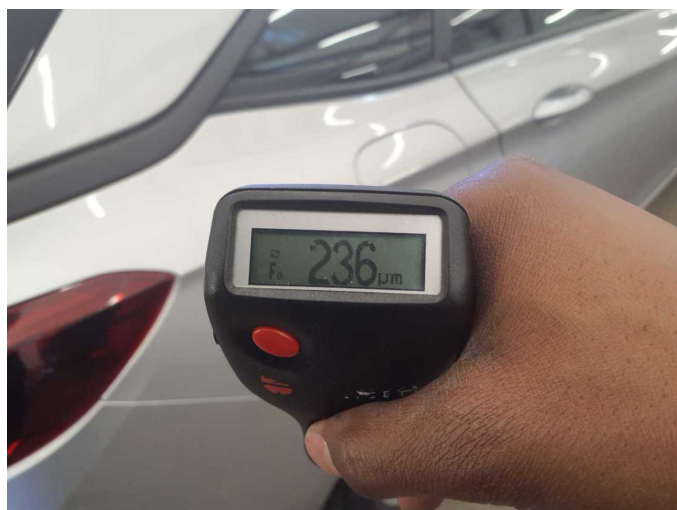
Repainting 8: Side panel - rear right side
