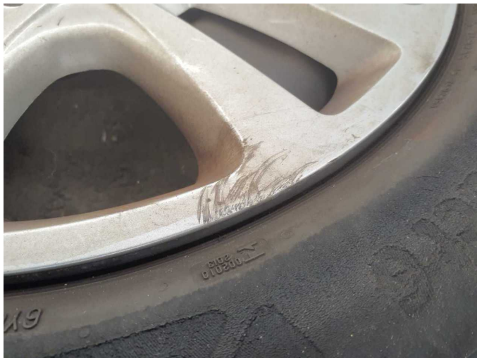
Damage 2: 2nd wheel set: 1 wheel cover - Scratched - Replace
