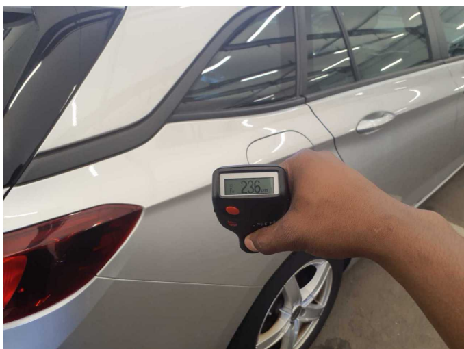
Repainting 8: Side panel - rear right side
