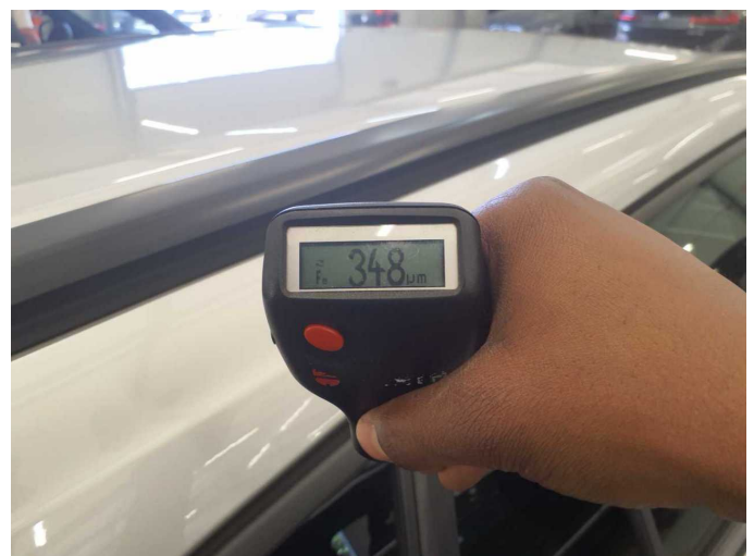
Repainting 3: Roof rail - right side
