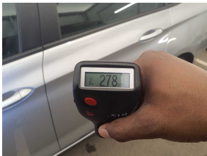
Repainting 9: Door - rear left side
