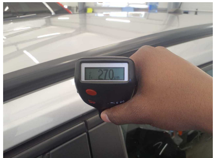
Repainting 2: Roof rail - left side
