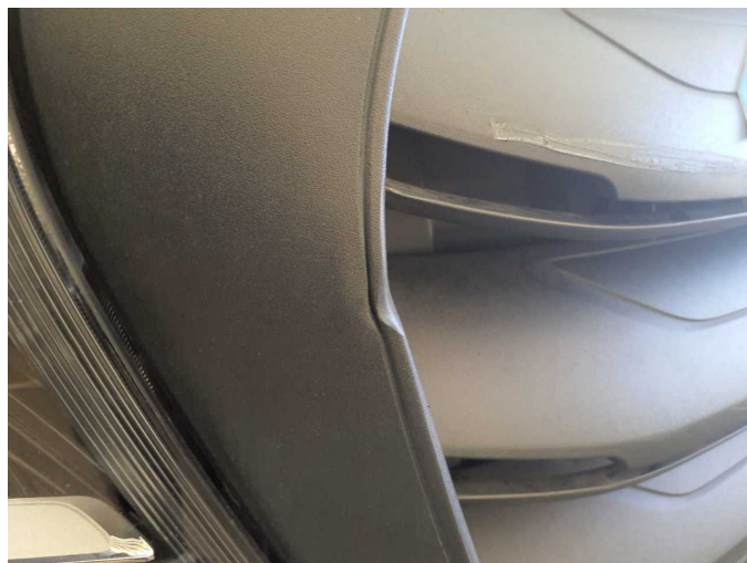
Damage 5: Bonnet: Radiator grille (+ verformt) - Scratched - Replace
