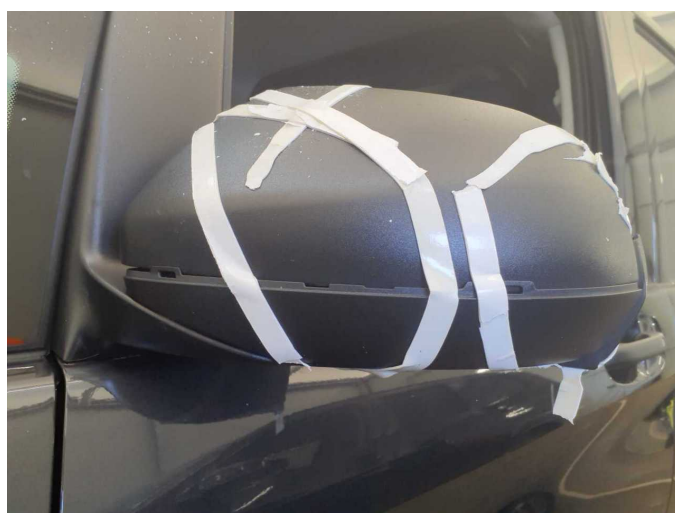
Damage 6: Wing mirror - left side: Wing mirror - Broken / torn - Replace
