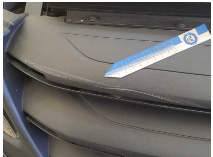
Damage 5: Bonnet: Radiator grille (+ verformt) - Scratched - Replace
