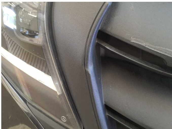
Damage 5: Bonnet: Radiator grille (+ verformt) - Scratched - Replace
