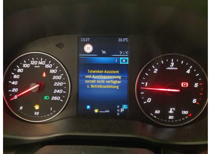
Damage 3: Instrument panel: Indicator light (Totwinkel Assistent) - Non-operational - Perform diagnosis
