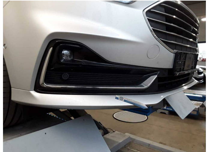
Damage 3: Front bumper: Front bumper - Scratch(es) - Smart repair
