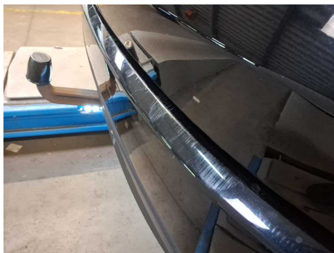
Damage 12: Rear bumper: Rear bumper - Scratched - Paint
