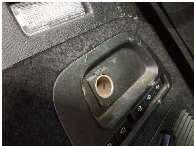
Damage 2: Electrical system: Power socket (12V) - Broken / torn - Loss in value
