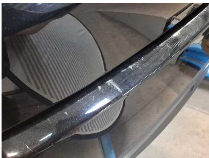
Damage 12: Rear bumper: Rear bumper - Scratched - Paint
