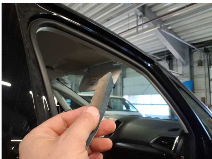
Damage 6: Interior: Sun visor - right side - Loose - Replace
