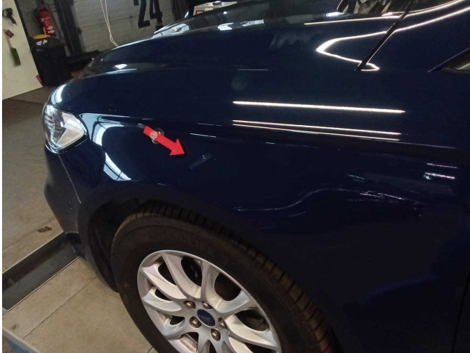
Damage 7: Mudguard - left side: Mudguard - left side - Scratched - Paint
