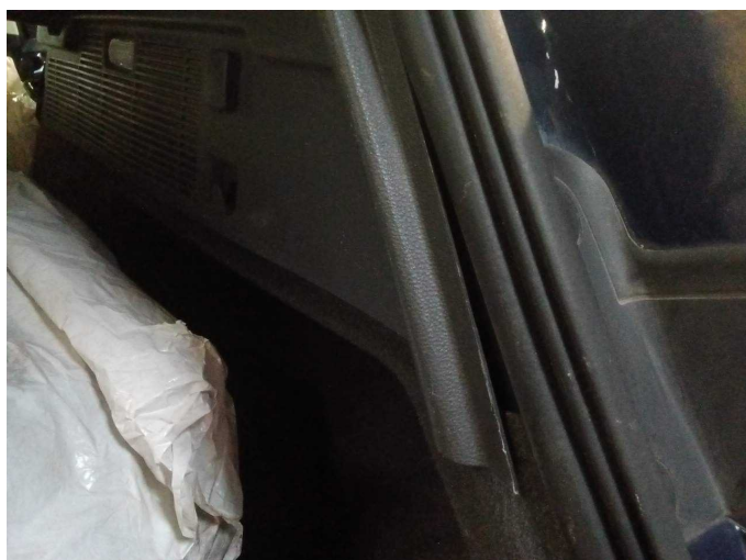
Damage 1: Trim / covers: Boot lining - Malposition - Un- / install
