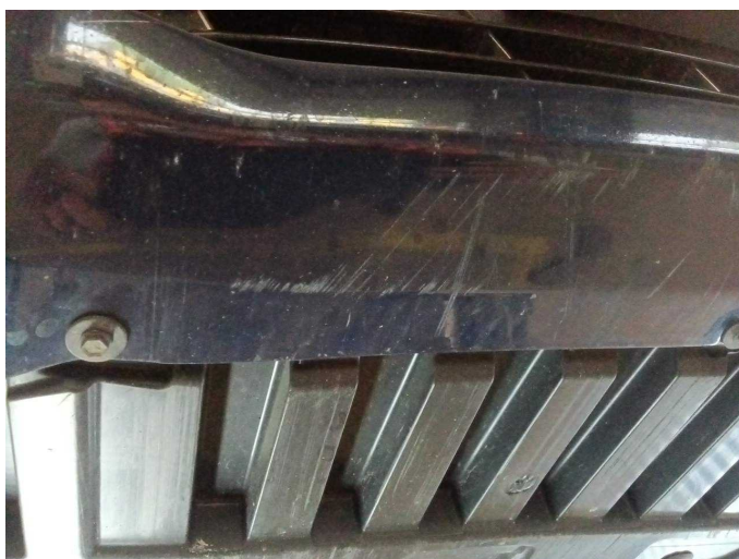
Damage 11: Front bumper: Front bumper - Scratched - Paint
