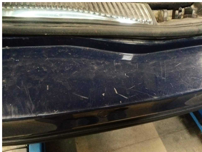
Damage 8: Rear bumper: Rear bumper - Scratched - Paint
