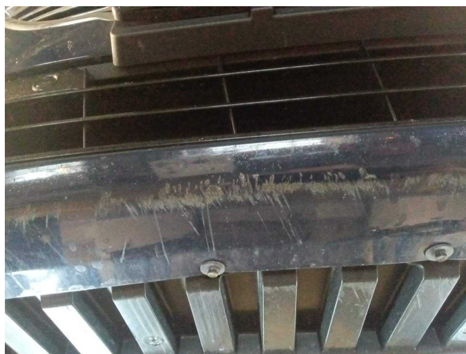
Damage 11: Front bumper: Front bumper - Scratched - Paint
