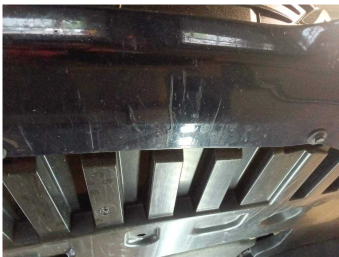
Damage 11: Front bumper: Front bumper - Scratched - Paint
