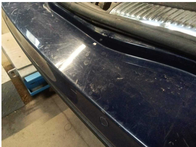
Damage 8: Rear bumper: Rear bumper - Scratched - Paint
