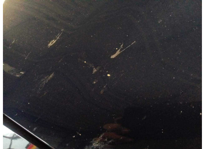
Damage 12: Bonnet: Bonnet - Dent / paintcoat damage - Paint
