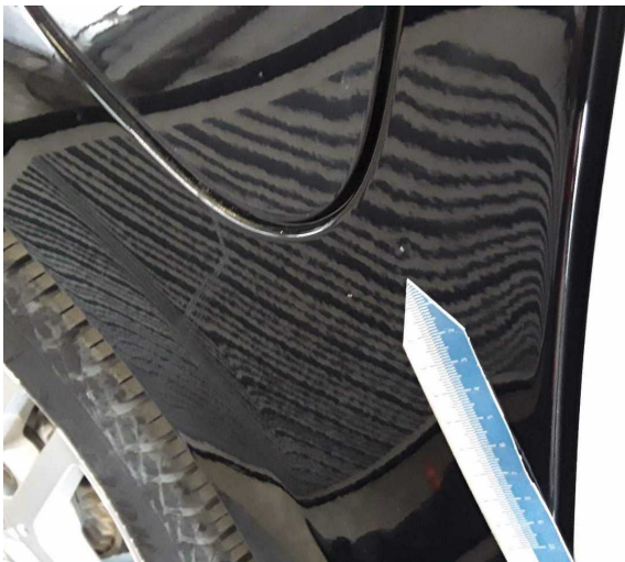
Damage 1: Side panel - rear right side: Side panel - dent(s) - Smooth repair work
