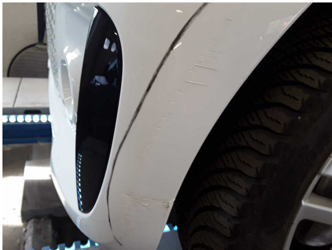
Damage 3: Front bumper: Front bumper - Scratched - Paint
