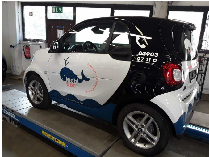
Damage 2: Body: Body - Glued / labelled - De-glue / neutralise
