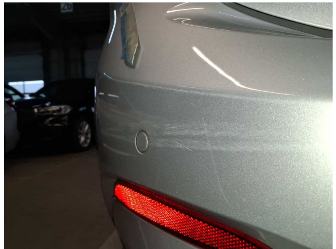
Damage 6: Rear bumper: Rear bumper - Scratched - Paint
