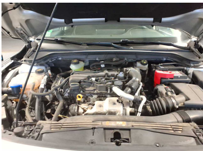
Missing part 1: Engine: Engine cover - Missing - Replace
