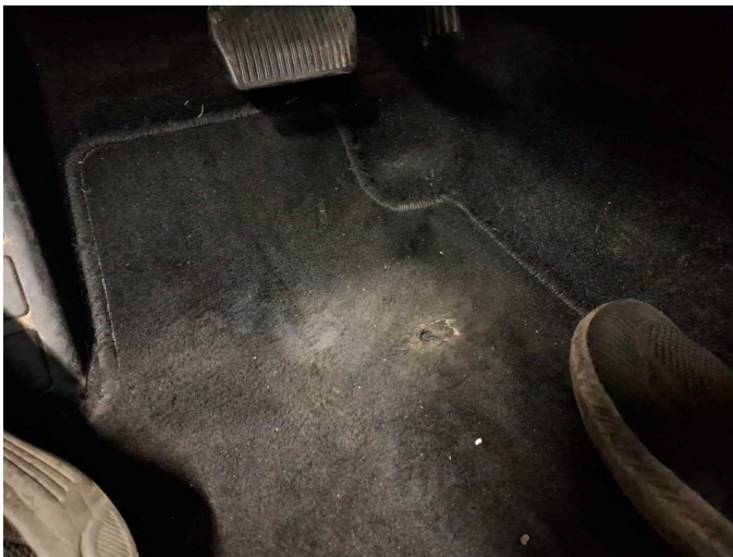
Damage 2: Trim / covers: Floor mats - Broken / torn - Replace
