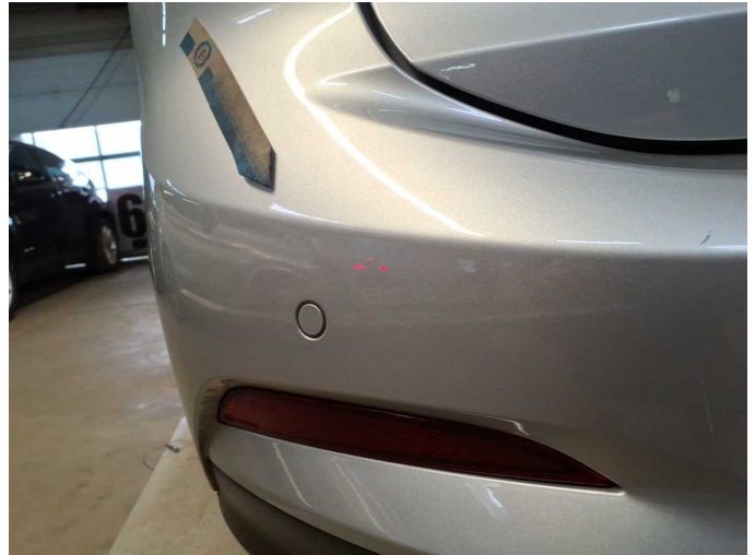
Damage 6: Rear bumper: Rear bumper - Scratched - Paint
