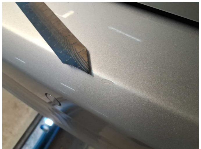
Damage 6: Rear bumper: Rear bumper - Scratched - Paint
