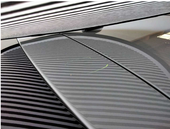
Wear and tear 1: Boot lid / rear door: Boot lid - dent(s) - No deduction
