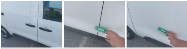
Door trim RR, Scratch(es), Repair and paint (complete)
