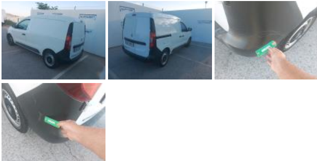
Boot door panel RR, Dent(s), Repair and paint (complete)
