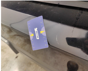
Bumper Front // Smart Repair Large-scratch
