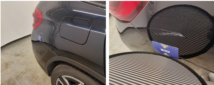
Wing Rear Right // Repair & Painting-scratch + dent
