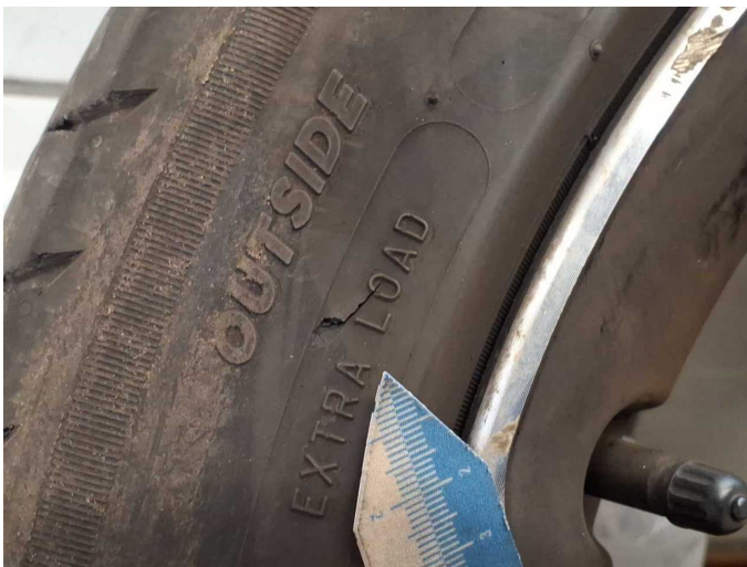
Damage 8: 2nd wheel set: 1 tyre - Broken / torn - Replace
