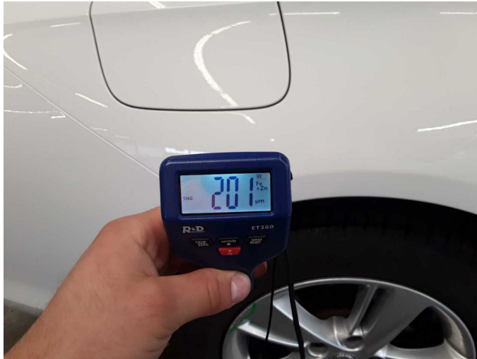
Side panel - rear right side: 201 µm
