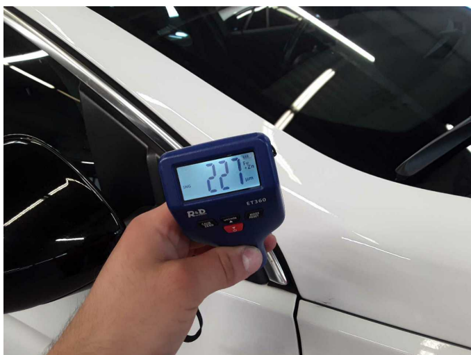
Roof rail - right side: 227 µm
