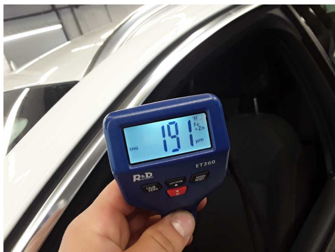
Roof rail - left side: 191 µm
