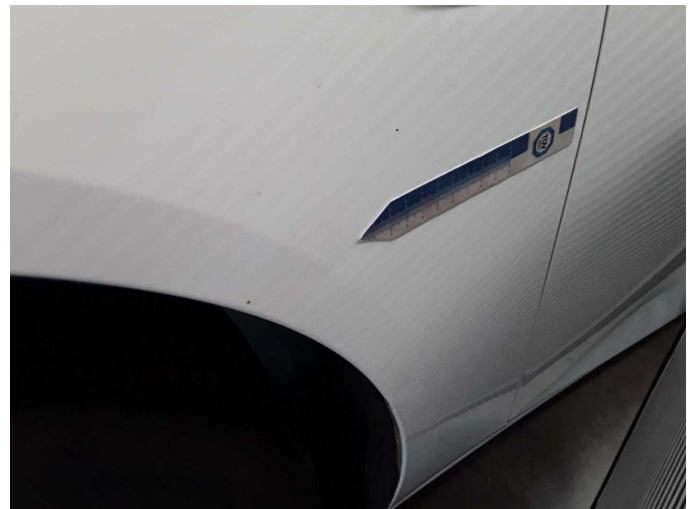
Damage 6: Mudguard - left side: Mudguard - left side - dent(s) - Repair and paint
