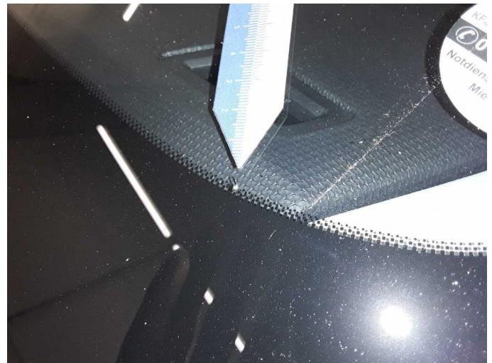
Damage 8: Vehicle glazing: Windscreen - Stone chips - Replace
