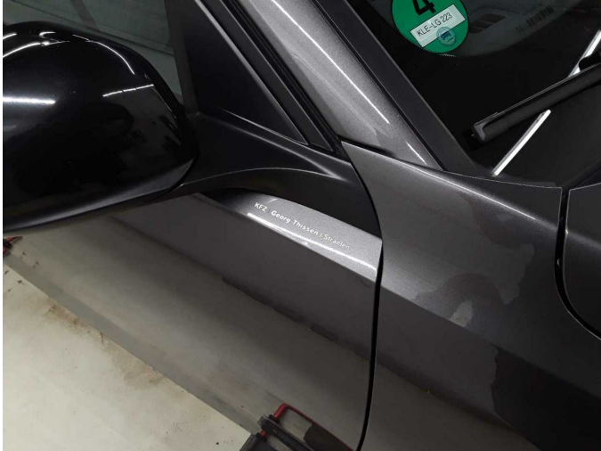
Damage 2: Body: Body - Glued / labelled - De-glove / neutralise
