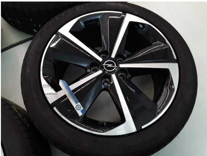
Damage 3: 2nd wheel set: 1 alloy rim - Scratched - Replace
