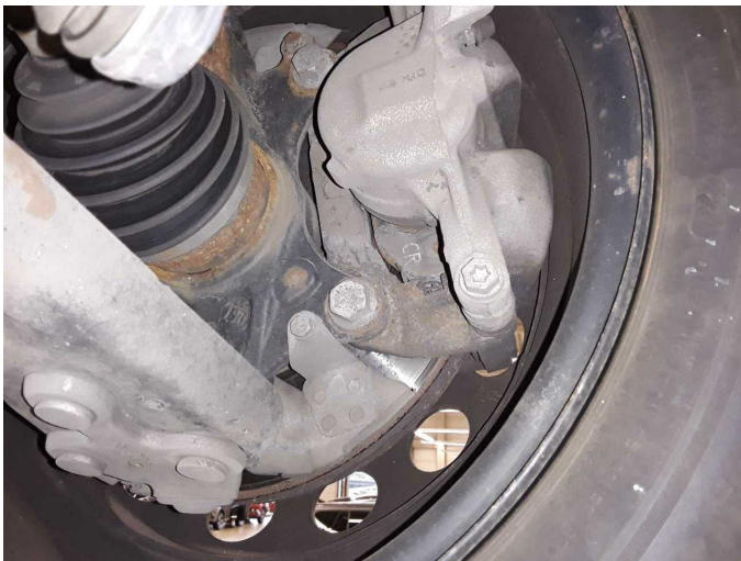
Damage 7: Braking system: Brake discs and brake pads - front (Korrosion und) - Worn - Replace
