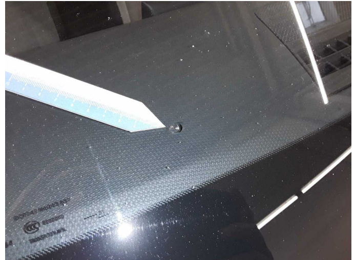
Damage 8: Vehicle glazing: Windscreen - Stone chips - Replace
