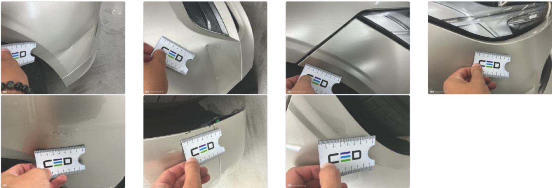
7 - Wing FR - Bad repair
