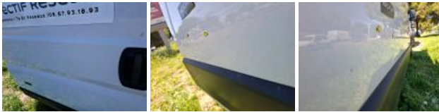
Side panel moulding R, Deformed / Strained, Replace
