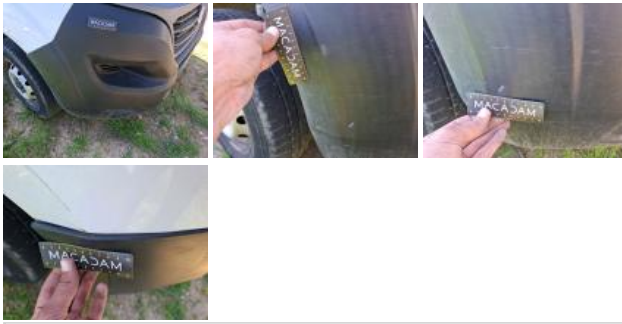
Bumper grille, Broken, Replace
