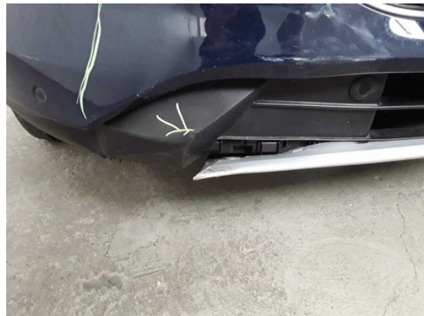
Damage #11: Front bumper: Spoiler - Deformed - Replace
