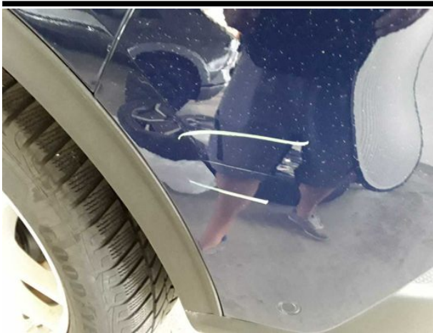
Damage #15: Rear bumper: Rear bumper - Scratched - Paint
