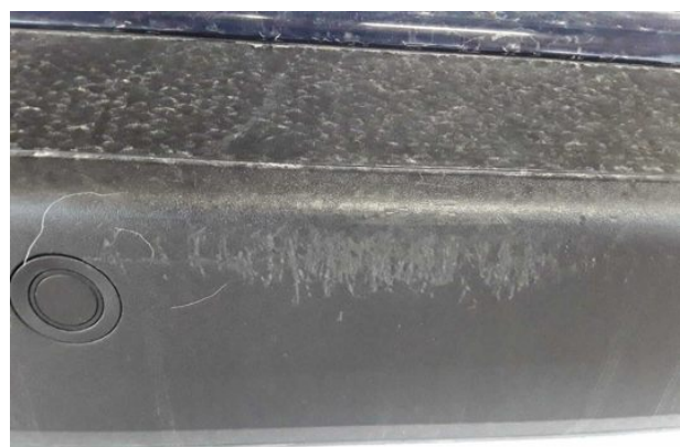
Damage #11: Front bumper: Spoiler - Deformed - Replace
