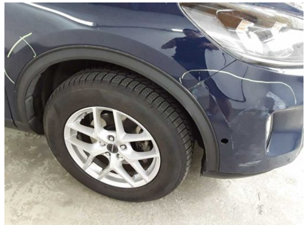
Damage #3: Mudguard - right side: Wheel well extension - Scratched - Loss in value
