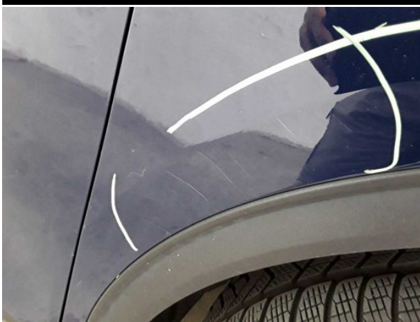
Damage #14: Mudguard - right side: Mudguard - right side - Dent / paintcoat damage - Repair and paint
