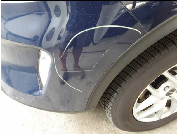
Damage #21: Front bumper: Front bumper - Deformed - Replace
