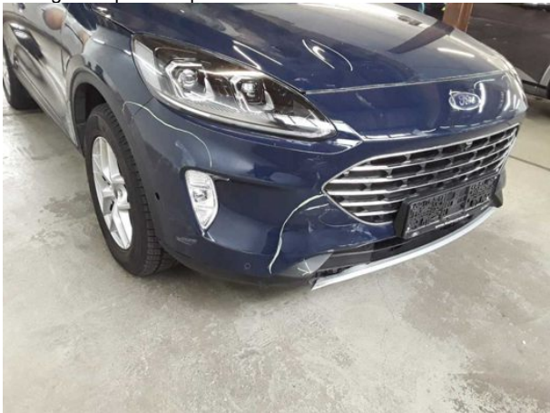
Damage #21: Front bumper: Front bumper - Deformed - Replace
