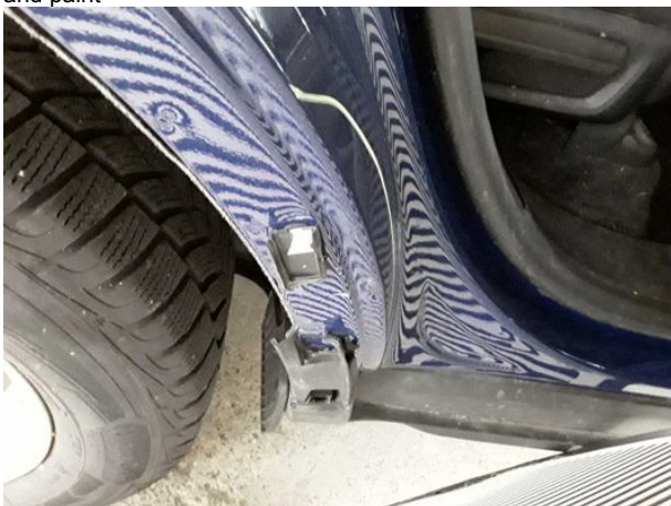
Damage #13: Side panel - rear right side: Sill - Deformed - Repair and paint
