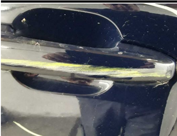
Damage #10: Door - rear right side: Door handle - outside - Scratched - Replace
