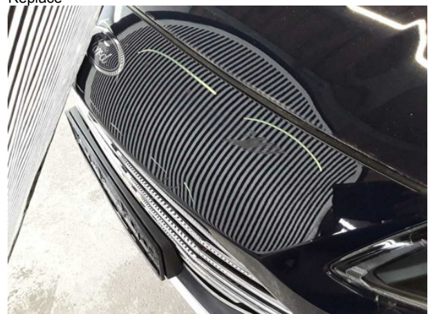
Damage #21: Front bumper: Front bumper - Deformed - Replace
