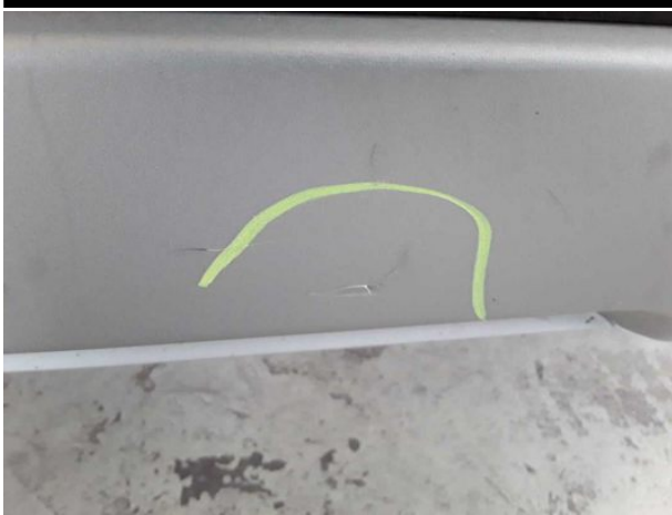
Damage #12: Rear bumper: Spoiler - Scratched - Replace
