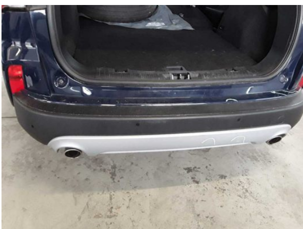
Damage #12: Rear bumper: Spoiler - Scratched - Replace
