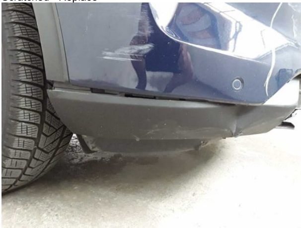
Damage #11: Front bumper: Spoiler - Deformed - Replace
