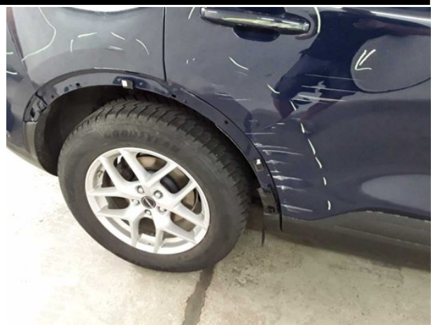
Damage #8: Side panel - rear right side: Wheel well extension... Broken / torn - Replace
