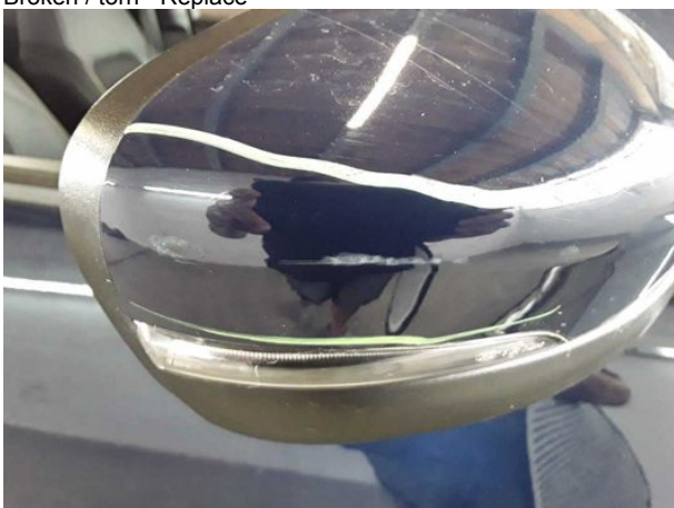
Damage #9: Wing mirror - right side: Cap - Scratched - Paint
