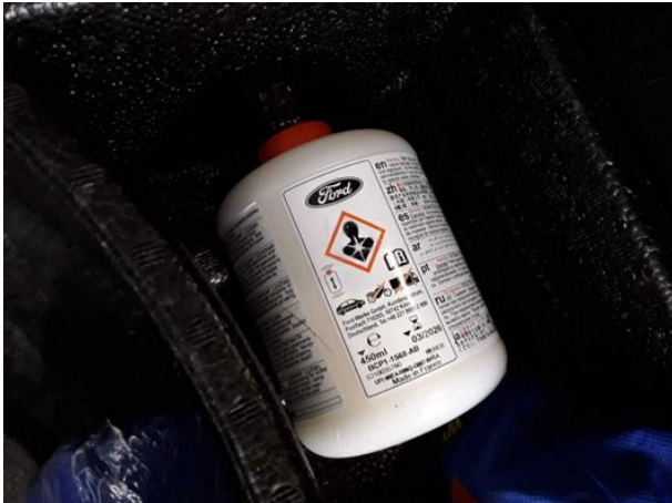
Damage #1: Equipment: Tirefit filler - Expired - Replace
