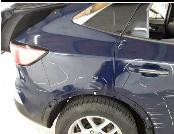
Damage #18: Side panel - rear right side: Side panel - Dent / paintcoat damage - Repair and paint
