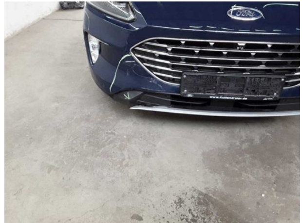
Damage #6: Front bumper: Air-inlet grille - Damaged - Replace
