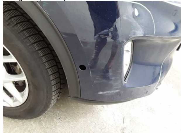
Damage #21: Front bumper: Front bumper - Deformed - Replace
