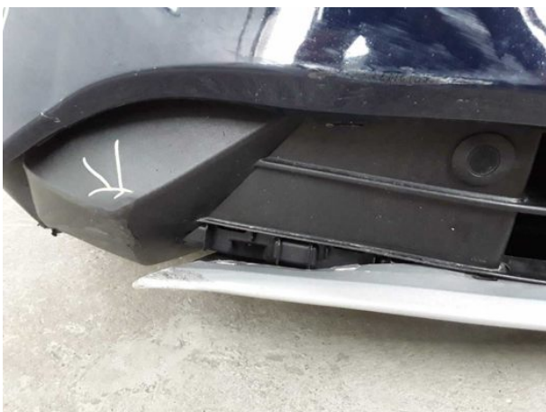
Damage #6: Front bumper: Air-inlet grille - Damaged - Replace
