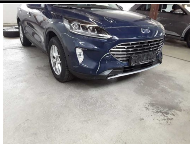
Damage #11: Front bumper: Spoiler - Deformed - Replace
