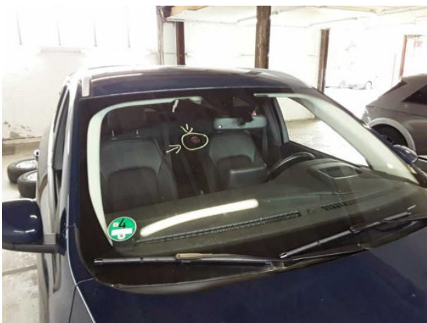
Damage #17: Vehicle glazing: Windscreen (Rissbildung) - Stone chips - Replace
