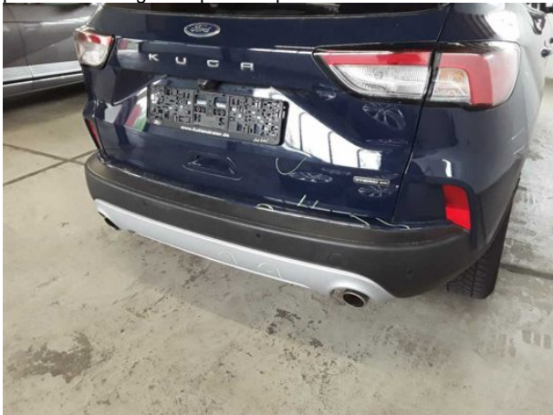
Damage #15: Rear bumper: Rear bumper - Scratched - Paint
