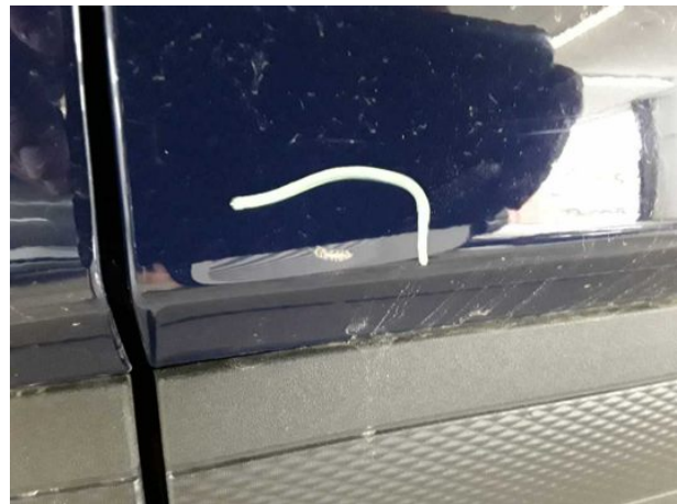
Damage #16: Door - rear left side: Door - Scratched - Paint
