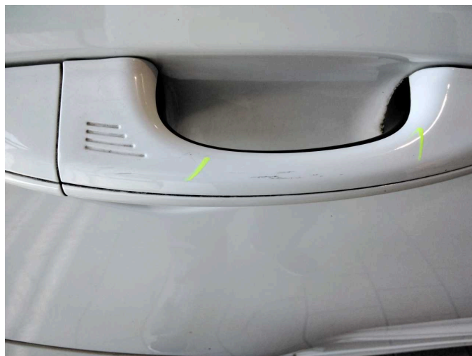
Damage 2: Door - rear right side: Door handle - outside - Scratch(es) - Smart repair
