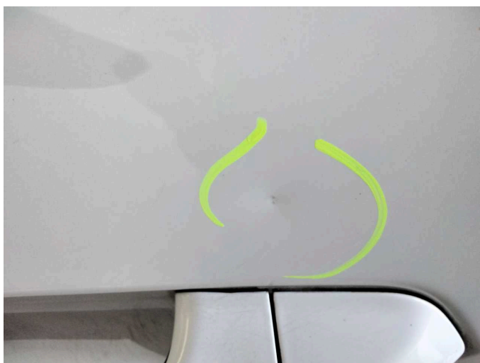
Damage 12: Door - front left side: Door - Dent / paintcoat damage - Paint
