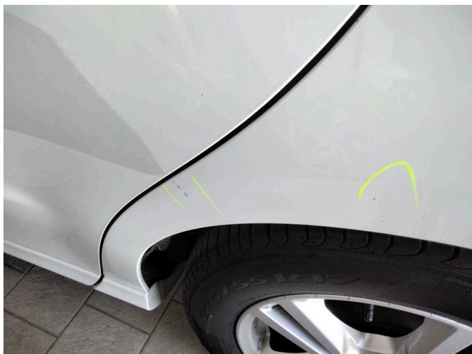
Damage 7: Side panel - rear left side: Side panel - Scratch(es) - Smart repair
