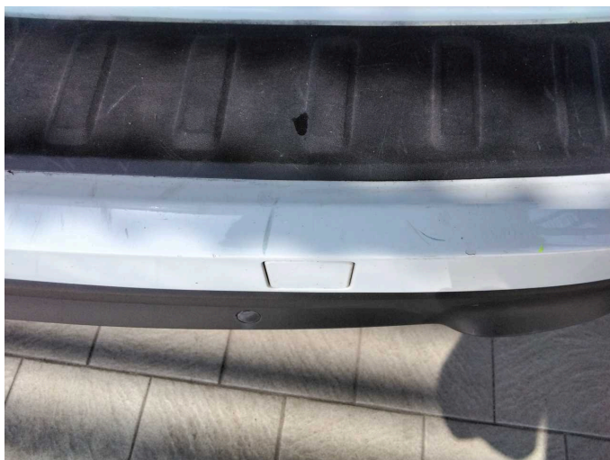
Damage 10: Rear bumper: Rear bumper - Scratch(es) - Paint
