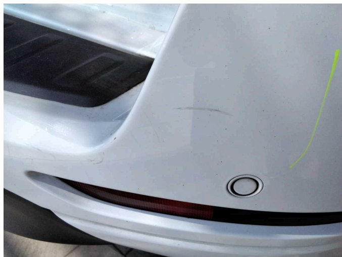
Damage 10: Rear bumper: Rear bumper - Scratch(es) - Paint
