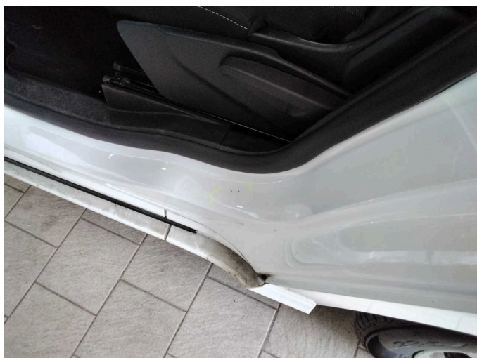
Damage 6: Body: C-pillar - left side - Dent / paintcoat damage - Smart repair
