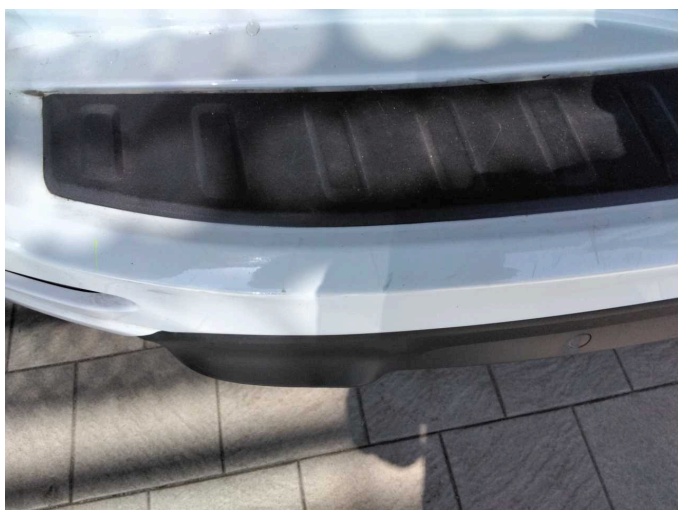
Damage 10: Rear bumper: Rear bumper - Scratch(es) - Paint
