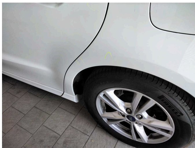
Damage 7: Side panel - rear left side: Side panel - Scratch(es) - Smart repair
