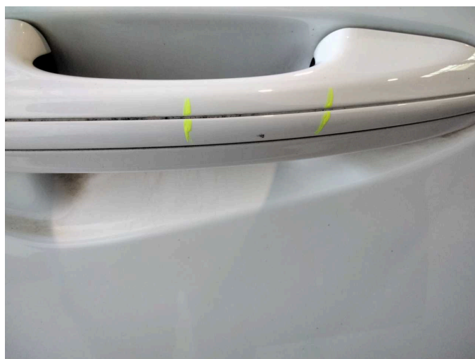
Damage 3: Door - front right side: Door handle - outside - Scratch(es) - Smart repair
