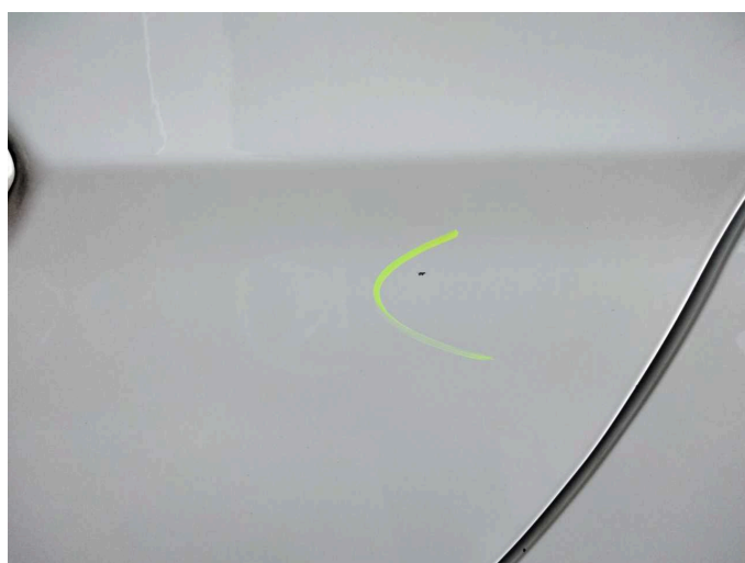
Damage 9: Door - rear left side: Door - Scratch(es) - Smart repair
