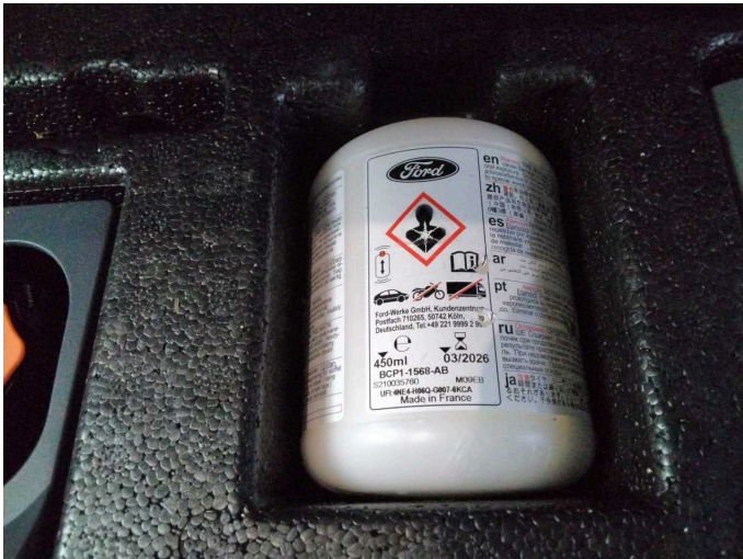
Damage 1: Equipment: Tirefit filler - Expired - Replace
