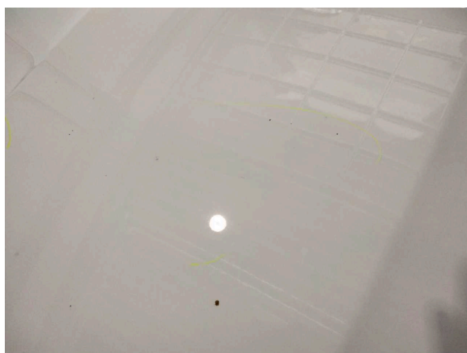
Damage 11: Bonnet: Bonnet - Stone chips - Paint
