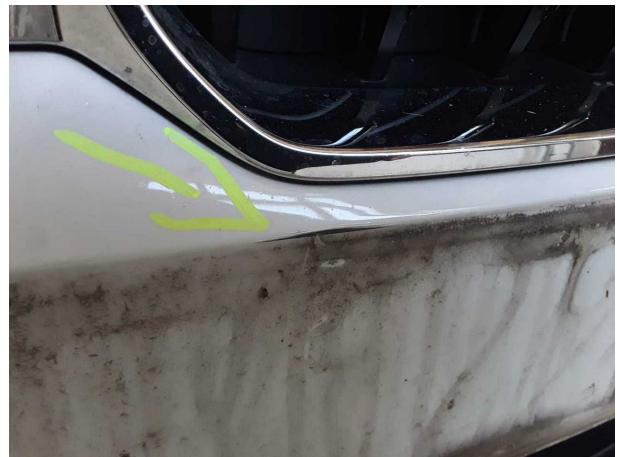
Damage #7: Front bumper: Front bumper - Deformed - Replace
