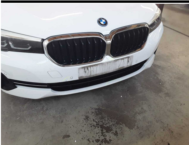
Damage #7: Front bumper: Front bumper - Deformed - Replace
