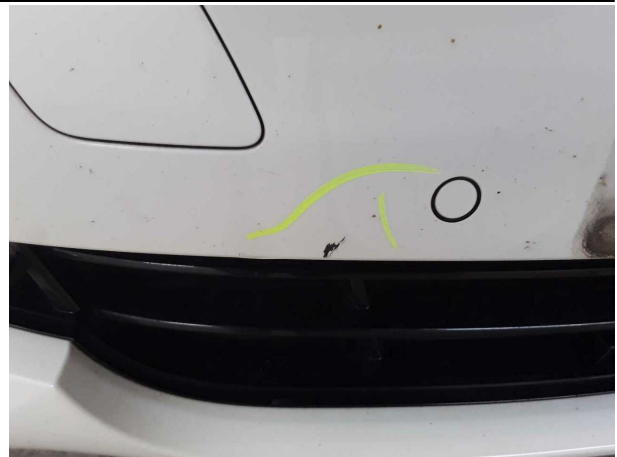
Damage #7: Front bumper: Front bumper - Deformed - Replace
