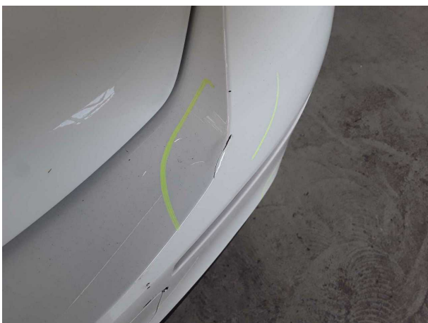
Damage #6: Rear bumper: Rear bumper - Deformed - Replace
