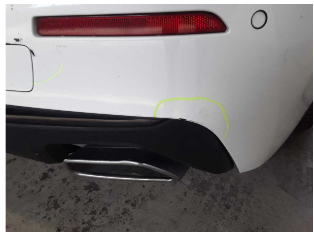
Damage #6: Rear bumper: Rear bumper - Deformed - Replace
