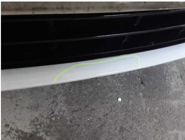
Damage #7: Front bumper: Front bumper - Deformed - Replace
