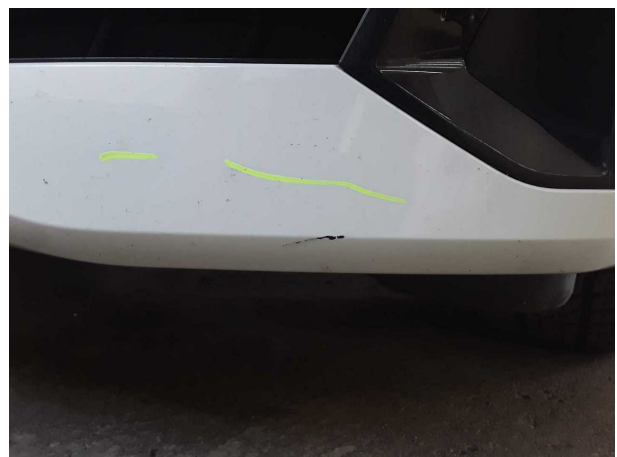
Damage #7: Front bumper: Front bumper - Deformed - Replace
