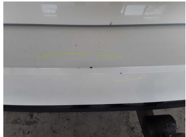
Damage #6: Rear bumper: Rear bumper - Deformed - Replace
