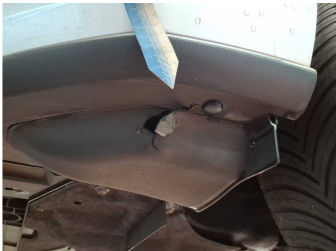
Damage 5: Body: Underbody panelling - Broken / torn - Replace
