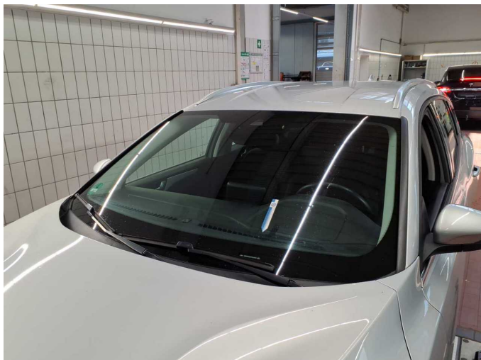
Damage 10: Vehicle glazing: Windscreen - Stone chips - Replace
