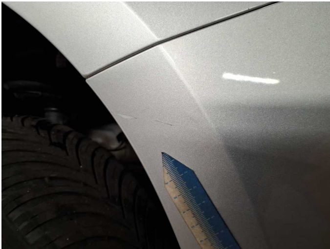
Damage 8: Front bumper: Front bumper - Scratch(es) - Paint
