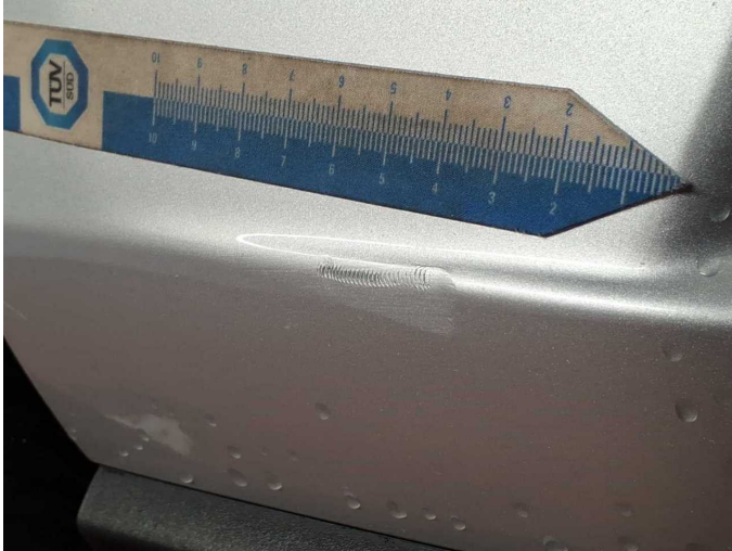
Damage 8: Front bumper: Front bumper - Scratch(es) - Paint
