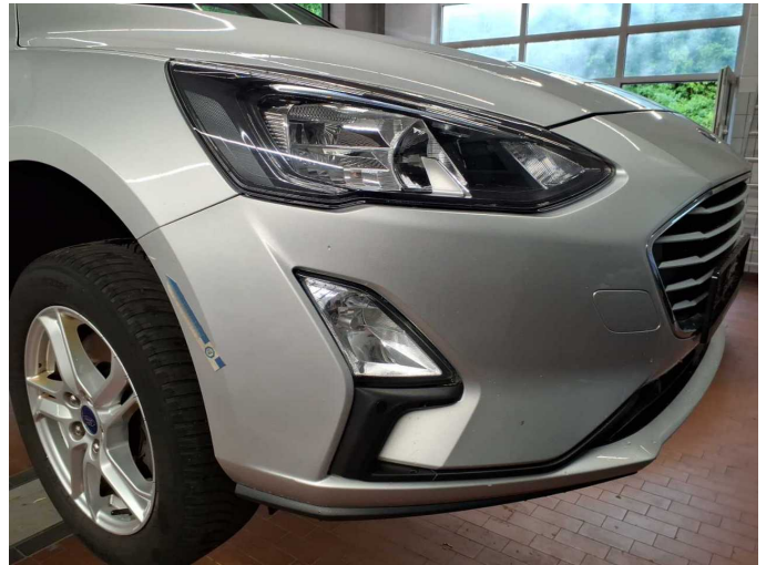
Damage 8: Front bumper: Front bumper - Scratch(es) - Paint
