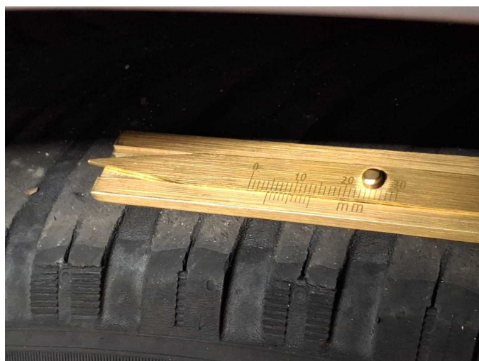
Damage 7: Wheel / tyres: Tyres - complete set (4mm) - Does not meet the leasing specifications - Replace
