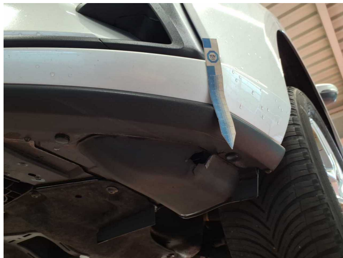
Damage 5: Body: Underbody panelling - Broken / torn - Replace
