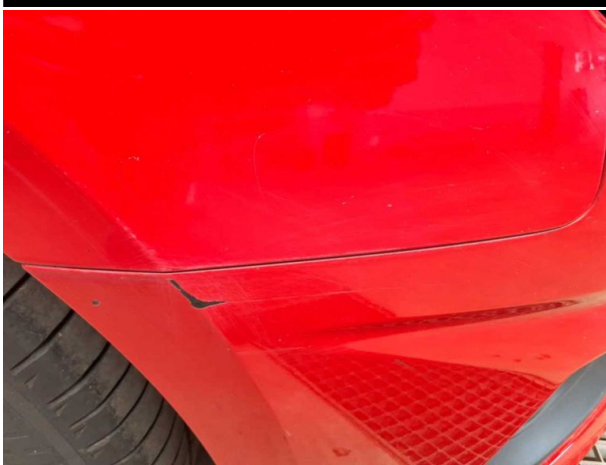
Damage #5: Mudguard - right side: Mudguard - right side - Scratch(es) - Paint
