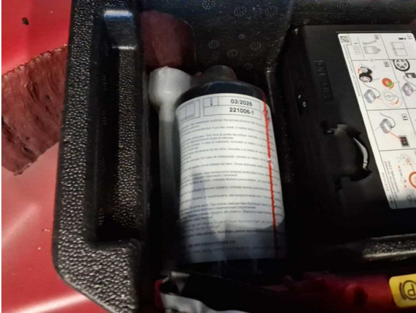
Damage #1: Equipment: Tirefit filler - Expired - Replace
