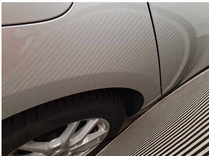
Damage 5: Side panel - rear right side: Side panel (3x) - dent(s) - Smooth repair work
