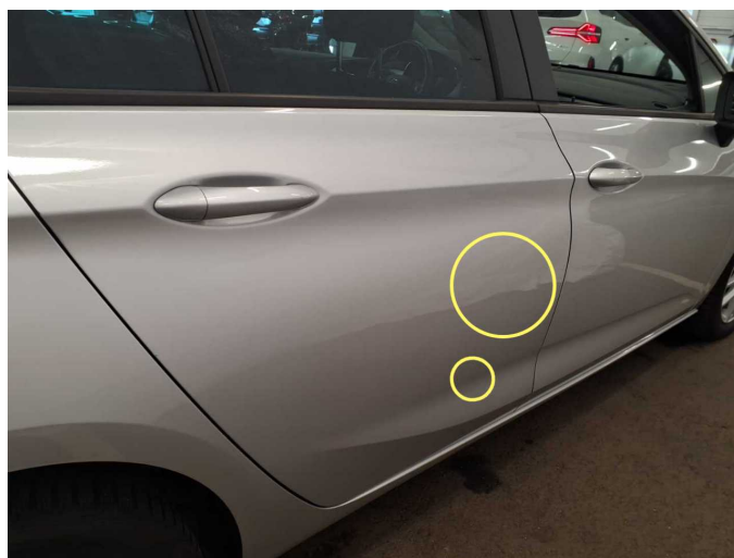
Damage 7: Door - rear right side: Door - Dent / paintcoat damage - Repair and paint
