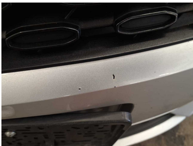
Damage 8: Front bumper: Front bumper - Scratch(es) - Paint
