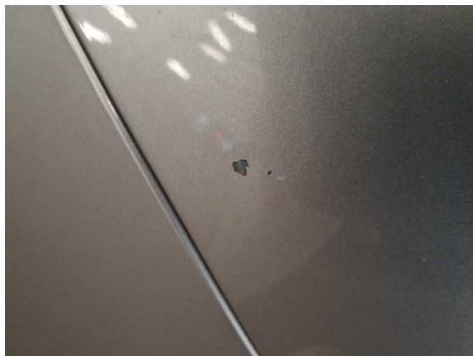
Damage 3: Mudguard - left side: Mudguard - left side - Stone chips - Smart repair
