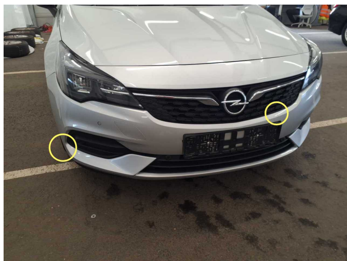
Damage 8: Front bumper: Front bumper - Scratch(es) - Paint
