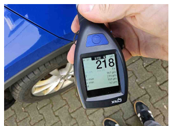
Paint thickness Roof
