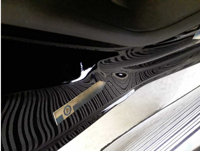
Damage 5: Side panel - rear right side: Elbow - dent(s) - Smooth repair work
