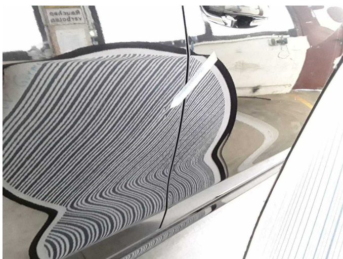
Damage 4: Door - rear right side: Door (2 Dellen nebeneinander) - dent(s) - Smooth repair work
