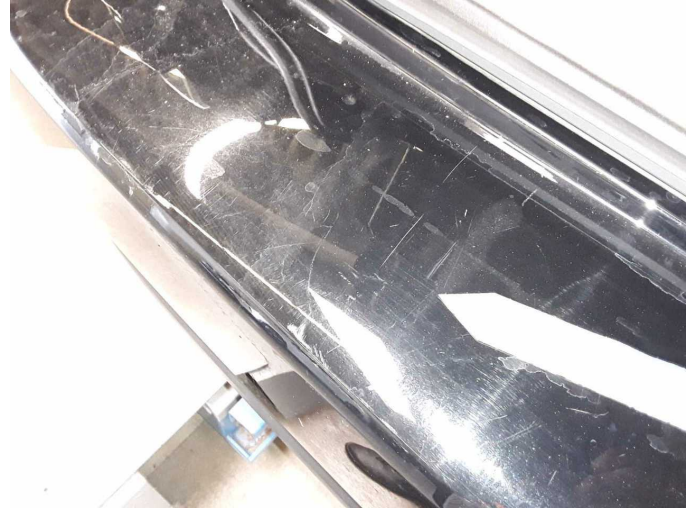
Damage 6: Rear bumper: Rear bumper - Scratch(es) - Paint
