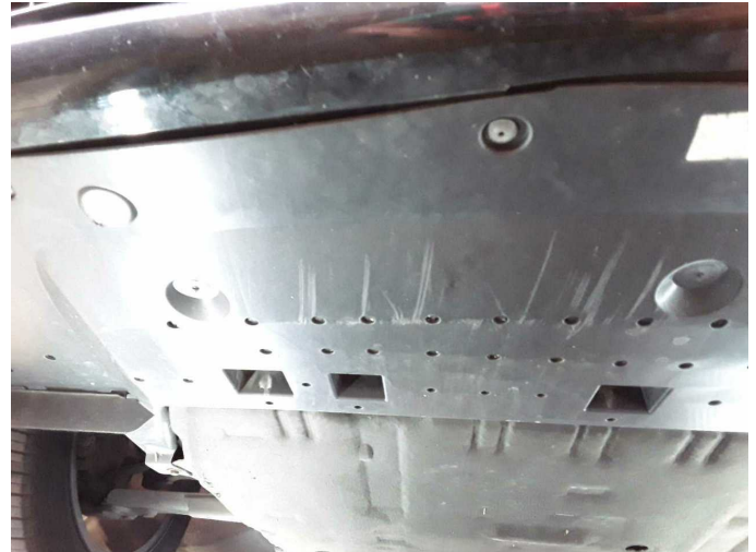
Damage 1: Body: Underbody panelling - Scratched - Loss in value
