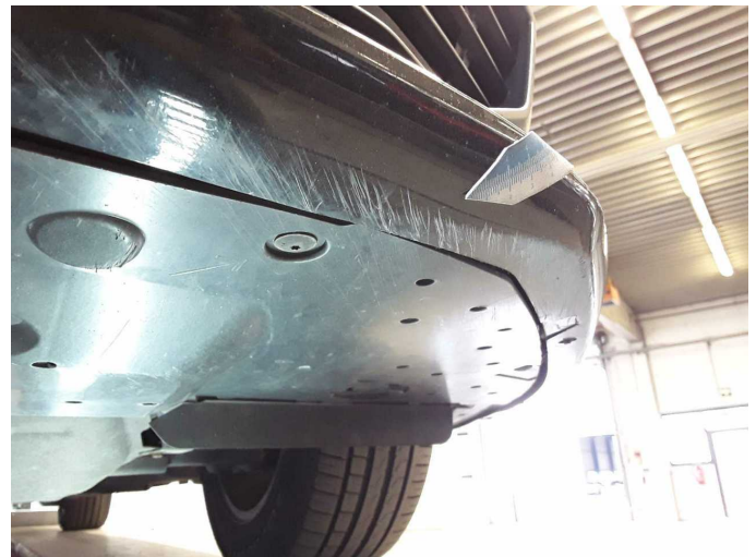
Damage 7: Front bumper: Front bumper - Scratched - Paint
