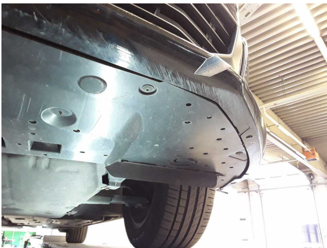
Damage 7: Front bumper: Front bumper - Scratched - Paint
