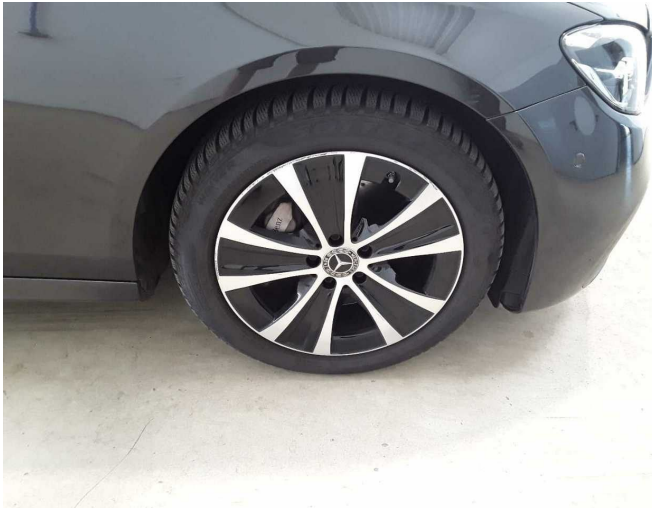
Damage 6: Wheel / tyres: Alloy rim - front right side - Scratch(es) - Replace
