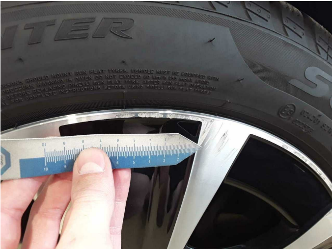
Damage 8: Wheel / tyres: Alloy rim - rear left side - Scratch(es) - Replace
