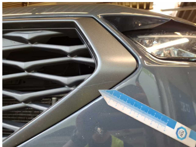
Damage 2: Front structure: Grille - Scratch(es) - Smart repair
