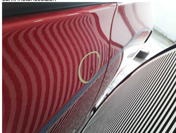
Beschädigung #2: Tür vorn links: Tür - Delle / Lackschaden - Smart Repair
