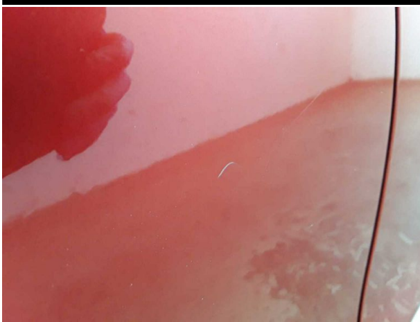
Damage #3: Door - rear right side: Door - Scratch(es) - Smart repair
