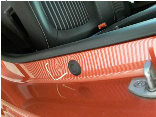
Damage #4: Side panel - rear left side: Sill - dent(s) - Smooth repair work
