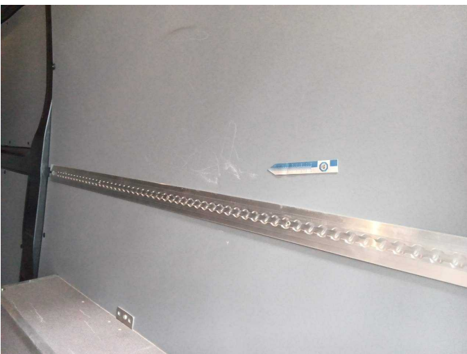
Damage 1: Side panel - rear right side: Interior trim - Scratched - Loss in value
