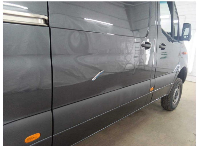
Damage 4: Sliding door, right: Sliding door - dent(s) - Smart repair
