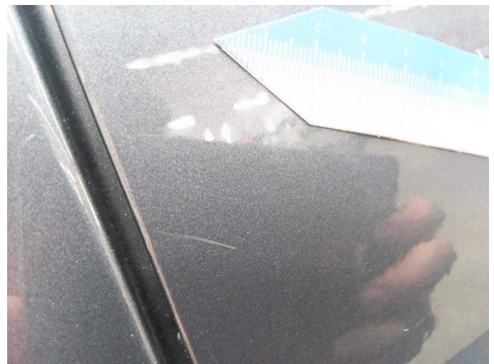
Damage 3: Boot lid / rear door: Rear door - right side - Scratch(es) - Smart repair
