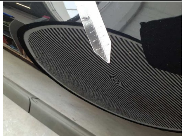
Damage #5: Door - rear left side: Door - dent(s) - Smooth repair work
