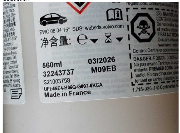
Damage #4: Equipment: Tirefit filler - Expired - Replace
