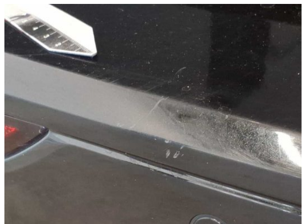
Damage #7: Rear bumper: Rear bumper - Scratch(es) - Smart repair
