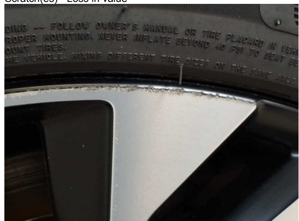
Damage #10: Wheel / tyres: Alloy rim - rear right side - Scratch(es) - Loss in value
