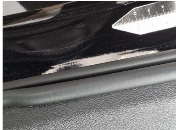
Damage #6: Sill - left side: Sill - Scratch(es) - Smart repair
