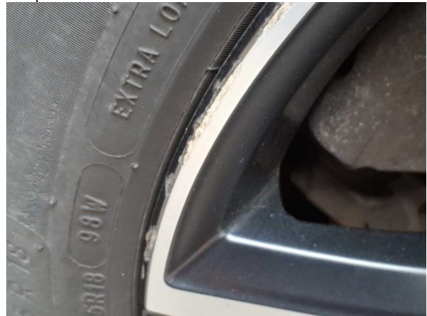
Damage #9: Wheel / tyres: Alloy rim - front left side - Scratch(es) - Loss in value
