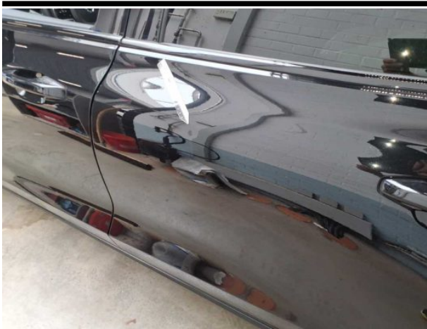
Damage #5: Door - rear left side: Door - dent(s) - Smooth repair work
