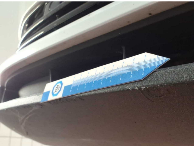
Damage 1: Front bumper: Spoiler - Scratch(es) - Replace
