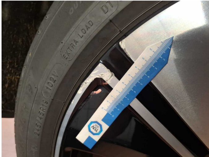
Damage 4: Wheel / tyres: Alloy rim - rear right side - Scratched - Replace
