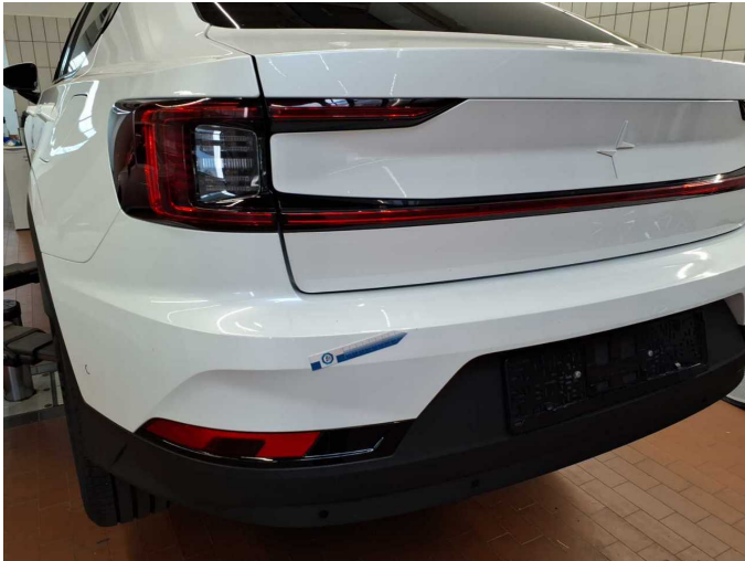
Damage 6: Rear bumper: Rear bumper - Scratch(es) - Paint
