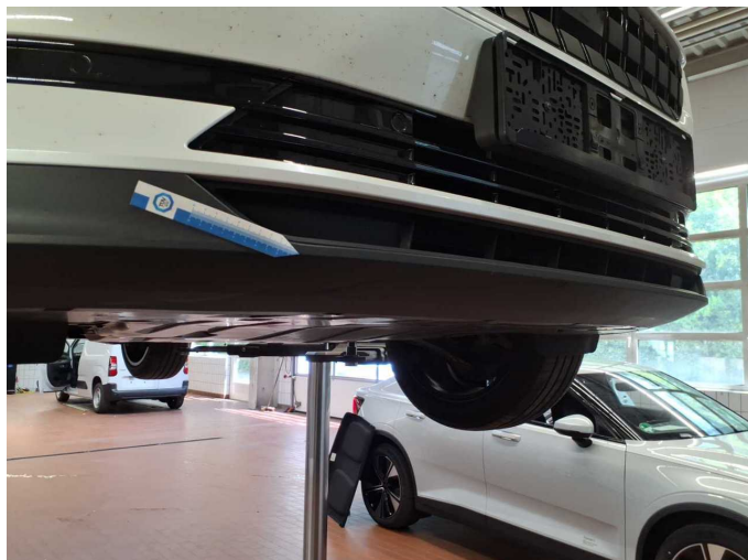
Damage 1: Front bumper: Spoiler - Scratch(es) - Replace
