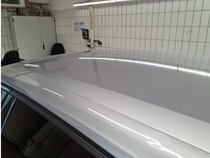
Damage 2: Roof: Roof - dent(s) - Smooth repair work
