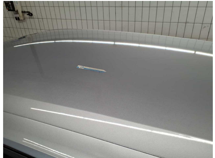
Damage 2: Roof: Roof - dent(s) - Smooth repair work
