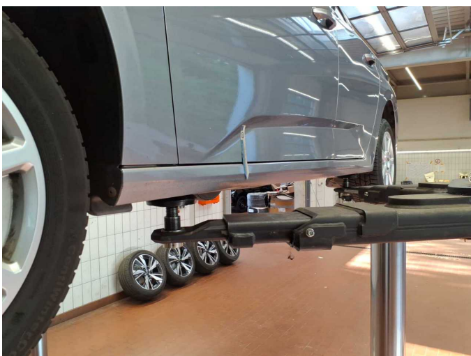
Damage 12: Sill - left side: Sill - Deformed - Repair and paint
