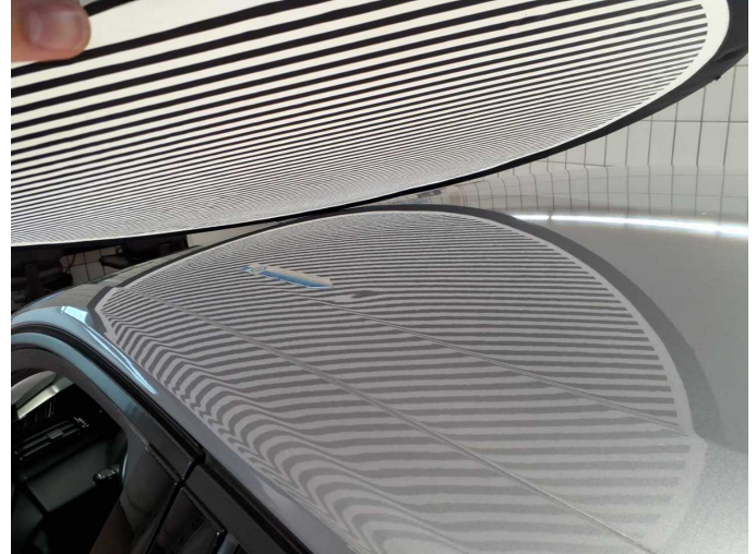
Damage 2: Roof: Roof - dent(s) - Smooth repair work
