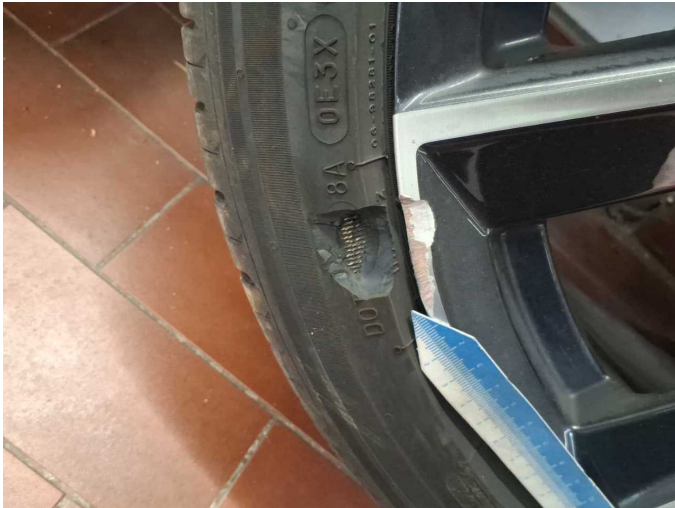
Damage 4: 2nd wheel set: 1 tyre - Broken / torn - Replace
