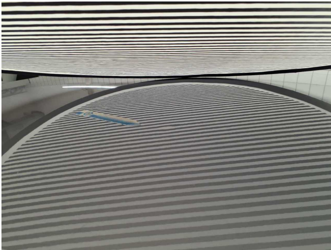
Damage 2: Roof: Roof - dent(s) - Smooth repair work
