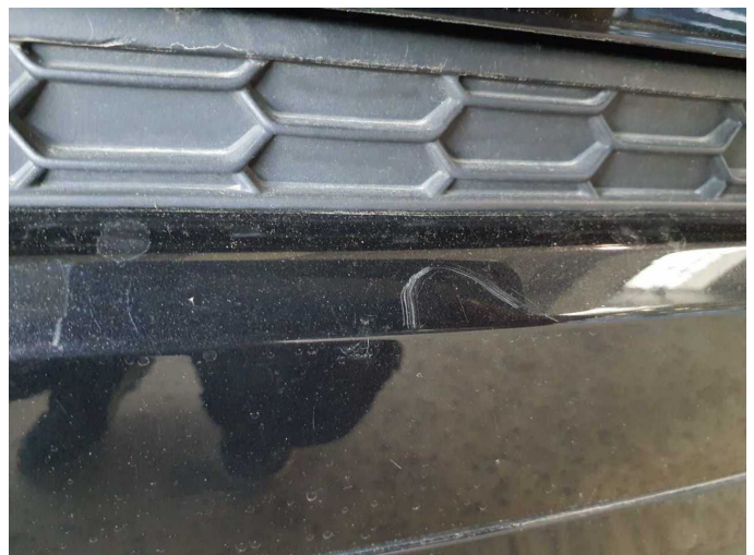
Damage 5: Rear bumper: Rear bumper - Scratch(es) - Paint
