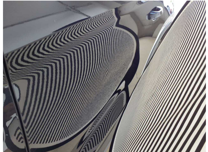
Damage 7: Door - rear left side: Door - Dent / paintcoat damage - Repair and paint
