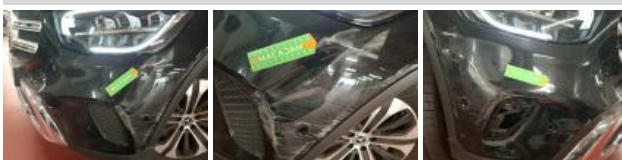
Bumper moulding FR, Missing, Replace
