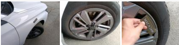
Tyre FR, Out of tolerance, Replace
