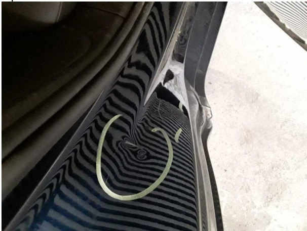
Damage #9: Side panel - rear right side: Sill - Dent / paintcoat damage - Repair and paint
