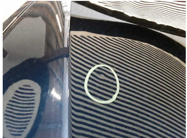
Damage #3: Bonnet: Bonnet - dent(s) - Smooth repair work
