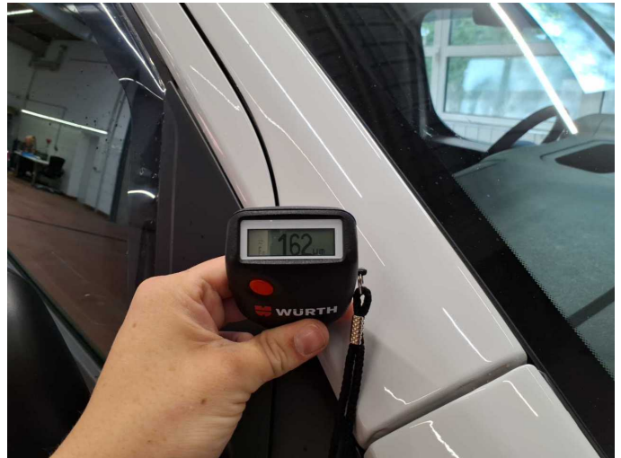
Repainting 1: Roof rail - right side
