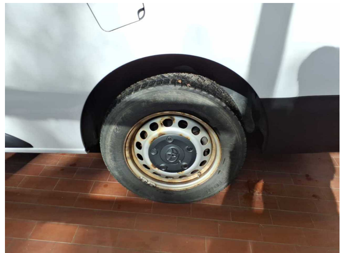
Damage 7: Wheel / tyres: Wheelset - complete (16 Zoll statt 17 Zoll) - Differs from the original configuration - Replace
