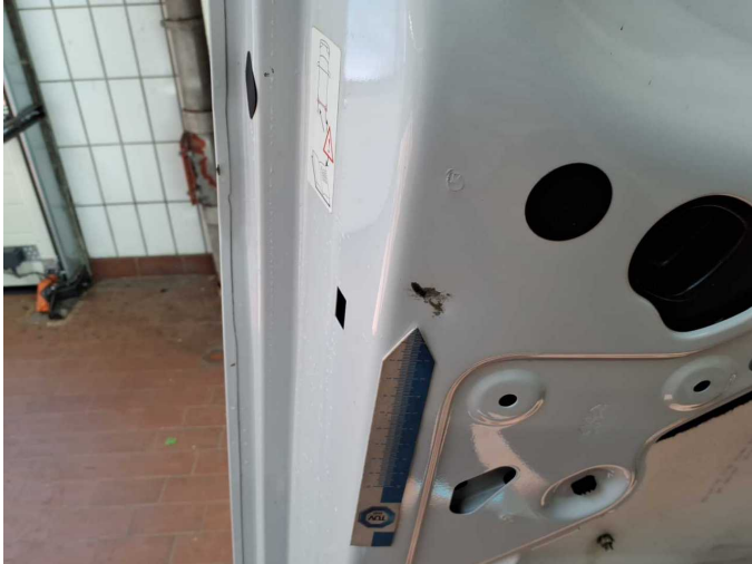
Damage 8: Boot lid / rear door: Rear door - left side (innen) - Dent / paintcoat damage - Repair and paint
