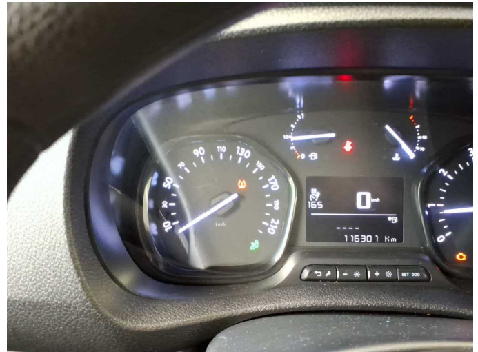
Damage 1: Instrument panel: Indicator light (Reifendruck) - on - Perform diagnosis
