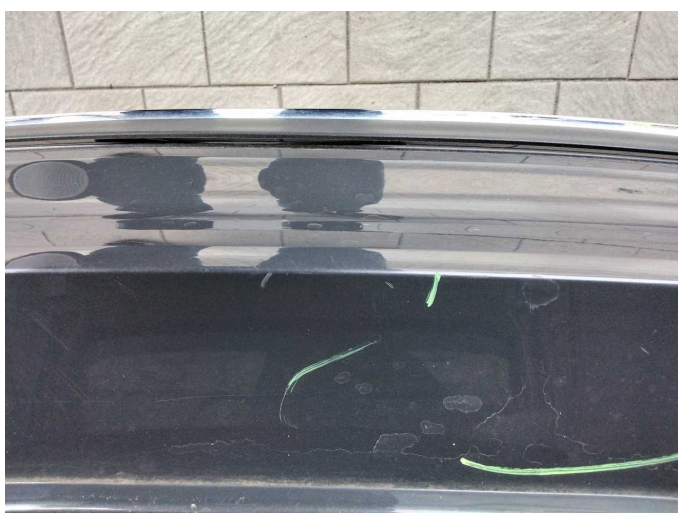
Damage 5: Rear bumper: Rear bumper - Dent / paintcoat damage - Repair and paint
