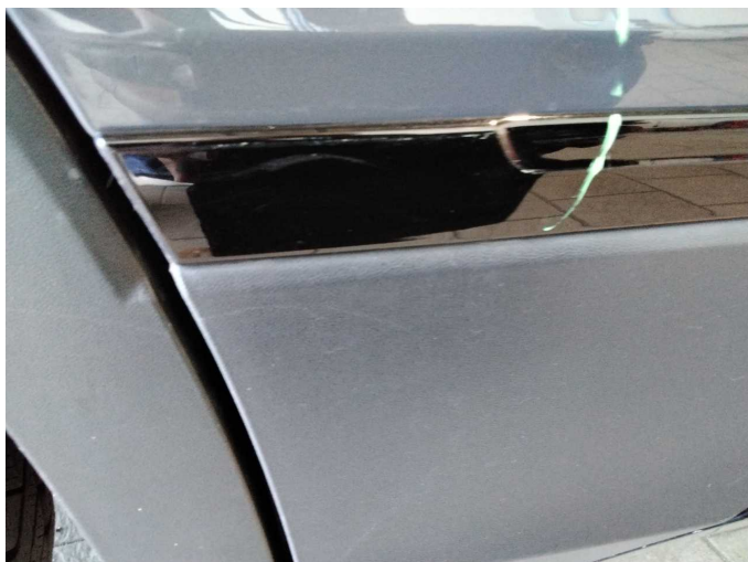
Damage 4: Door - rear right side: Brightware - lower - Scratch(es) - Replace
