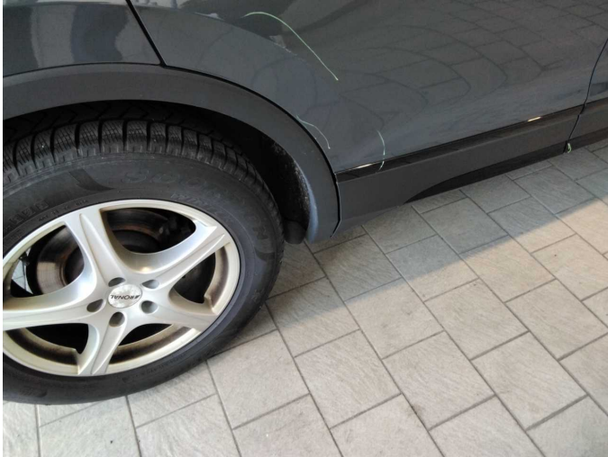
Wear and tear 5: Side panel - rear right side: Wheel well extension - Scratch(es) - No deduction
