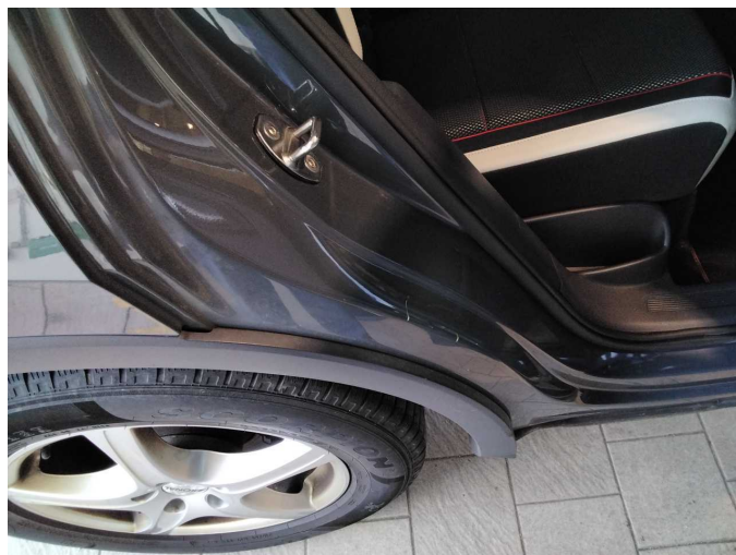
Damage 2: Body: C-pillar - right side - Scratch(es) - Smart repair
