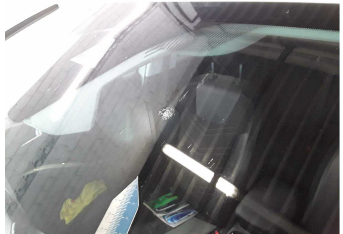
Damage 8: Vehicle glazing: Windscreen (Rissbildung) - Stone chips - Replace
