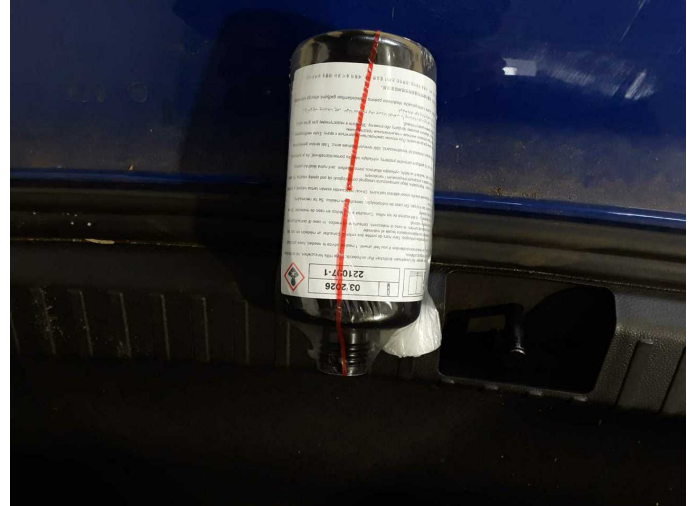
Damage 1: Equipment: Tirefit filler - Expired - Replace
