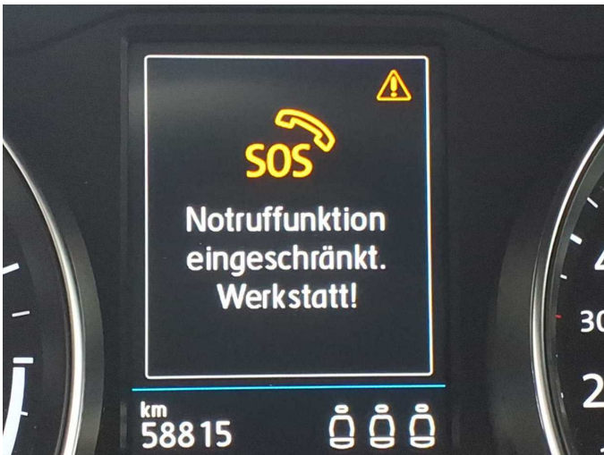
Damage 3: Electronic systems: Electronic systems (SOS-Notruf System) - Specify findings - Perform diagnosis
