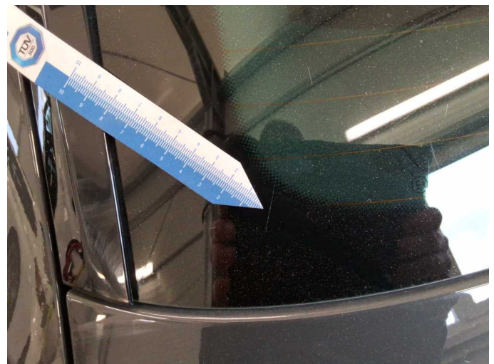
Damage 1: Vehicle glazing: Rear window (Im Randbereich) - Scratch(es) - Loss in value
