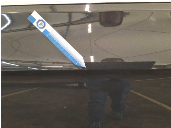
Wear and tear 3: Door - rear left side: Door - Scratch(es) - No deduction
