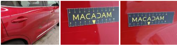
Door FR, Dent(s), Repair and paint (complete)
