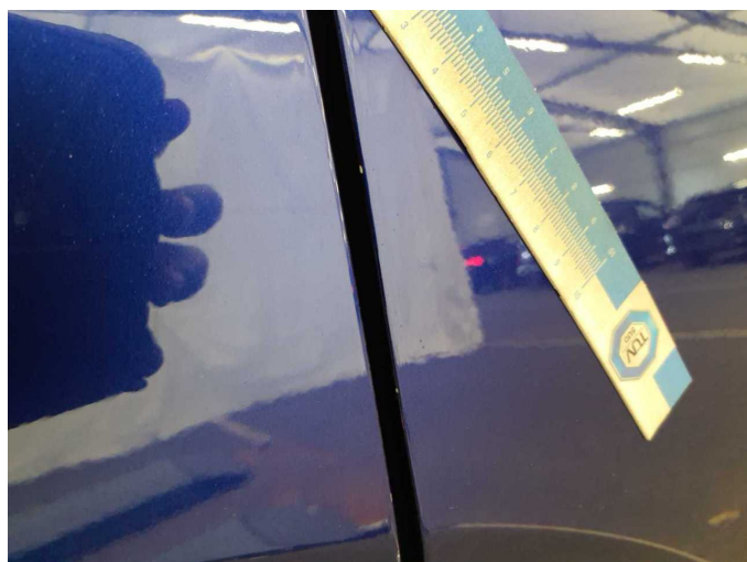
Damage 8: Door - rear right side: Door edge - Scratch(es) - Smart repair
