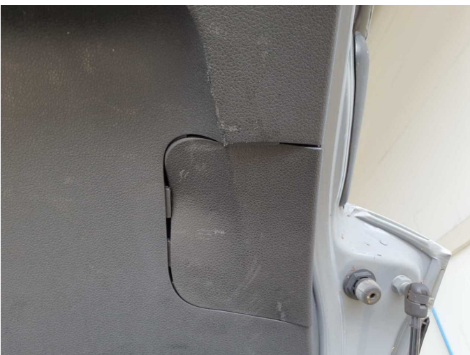
Damage 6: Boot lid / rear door: Trim - standard - lower (Abdeckkappe re.) - Deformed - Replace
