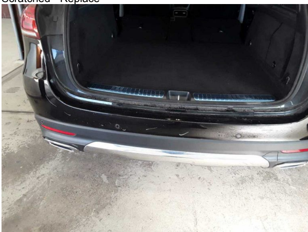
Damage #6: Rear bumper: Rear bumper - Scratched - Paint
