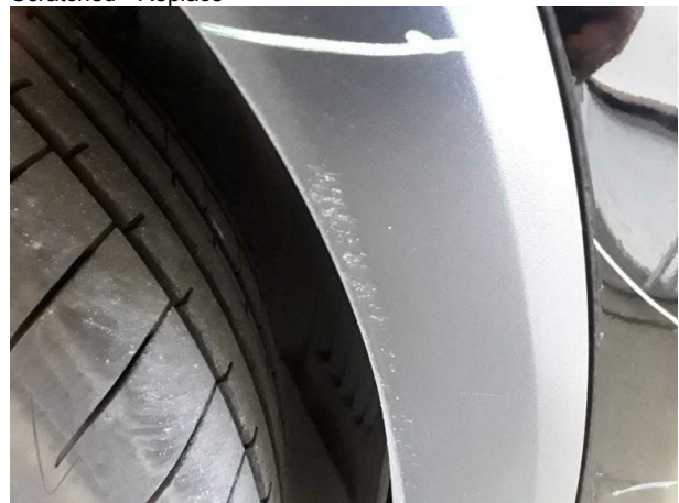
Damage #5: Mudguard - right side: Wheel well extension - Scratched - Replace
