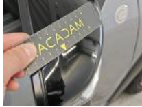
Outside rear-view mirror housing R, Scratch(es), Replace and paint
