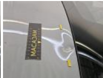
Roof, Dent(s), Repair and paint (complete)
