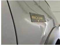
Outside rear-view mirror housing R, Scratch(es), Replace and paint
